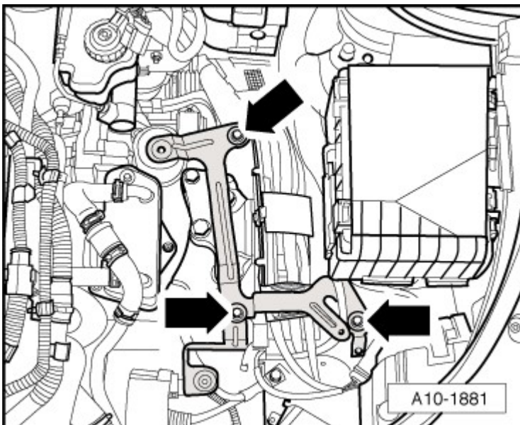
Fig. 10: Air Filter Housing Bracket Courtesy of AUDI OF AMERICA, LLC
