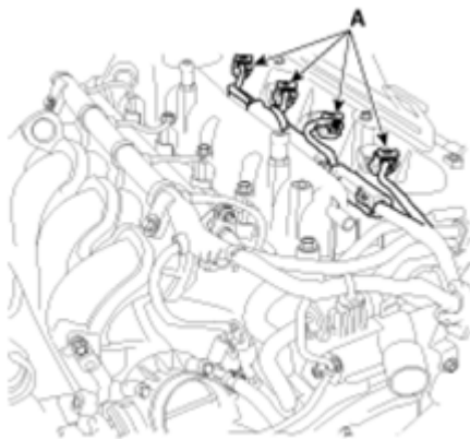
Fig. 9: Identifying Ignition Coil Connectors Courtesy of KIA MOTORS AMERICA, INC.
