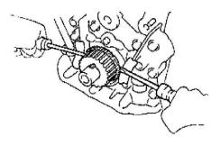
20. Remove crankshaft timing pulley.
