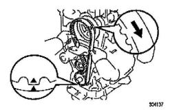
(a) Install the timing belt on the crankshaft timing pulley.
