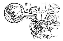
(a) Turn the crankshaft pulley and align its groove with the timing mark "0" of the No. 1 timing belt cover.
