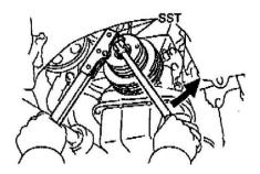
(a) Using Special Service Tool (SST) Crankshaft Pulley Holding Tool # 09213 - 54015 and Companion Flange Holding Tool # 09330 - 00021 or equivalents, remove the pulley bolt.
