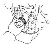
1. Install camshaft timing pulley.
