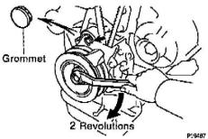
(a) Remove the grommet and loosen the timing belt idler pulley mounting bolt. (b) revolutions from TDC to TDC.
