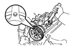
(a) Turn the hexagonal wrench head portion of the camshaft, and align the hole of the camshaft timing pulley with the timing mark of the bearing cap.
