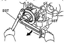
(b) Using Special Service Tool (SST) Crankshaft Pulley Holding Tool # 09213 - 54015, Companion Flange Holding Tool # 09330 - 00021 or equivalents, install the pulley bolt.
