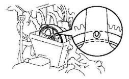
(b) Check that the hole of the camshaft timing pulley is aligned with the timing mark of the bearing cap. If not, turn the crankshaft one revolution  $(360^{\circ})$ .
