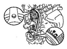
(c) Check that each pulley aligns with the marks as shown in the illustration.
