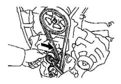
If the deflection is not as specified, readjust with the idler pulley.
