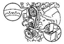
NOTE (When re-using timing belt): Place matchmarks on the timing belt to match the end of the No. 1 timing belt cover.
