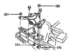
17. Install RH engine mounting insulator.
