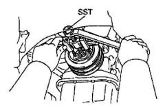
(b) Using SST Puller C Set # 09950 - 50010 (Hanger 150 # 09951 - 05010, Slide Arm # 09952 - 05010, Center Bolt 150 # 09953 - 05020, Claw No. 3 # 09954 - 05030) or equivalents, remove the pulley.
