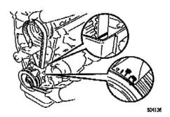
^ Check that the matchmark on the timing belt matches the end of No. 1 timing belt cover.
