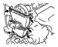
14. Remove No. 3 and No. 2 timing belt covers. Remove the 6 bolts and timing belt covers.
