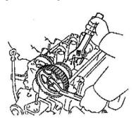
21. Remove camshaft timing pulley.
