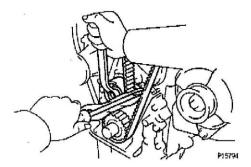
(a) Loosen the mounting bolt of the idler pulley and shift pulley toward the left as far as it will go and then temporarily tighten it. (b) Remove the belt.
