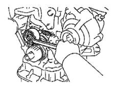
19. Remove idler pulley and tension spring. Remove the bolt, pulley and tension spring.
