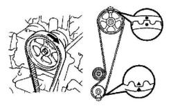
NOTE: If reusing the timing belt, draw a direction arrow on the belt (in the direction of engine revolution), and place matchmarks on the pulleys and belt as shown in the illustration.
