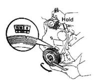
^ After aligning the matchmark, hold the timing belt. And turn the crankshaft pulley counterclockwise, and align its groove with timing mark "0" of the No.1 timing belt cover.
