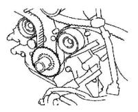
5. INSTALL TIMING BELT GUIDE Install the belt guide, facing the cup side outward. 6. INSTALL NO.1 TIMING BELT COVER
