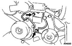
20. INSTALL NO.2 TIMING BELT COVER Install the No.2 timing belt cover with the 2 bolts. Torque: 16 Nm (160 kgf-cm, 12 ft. lbs.)
