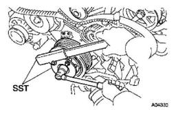
17. TIGHTEN CRANKSHAFT PULLEY BOLT Using SST, install the pulley bolt.
