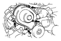
10. REMOVE RH NO.3 TIMING BELT COVER Remove the 3 bolts,nut RH No.3 timing belt cover.
