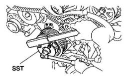
LOOSEN CRANKSHAFT PULLEY BOLT Using SST, loosen the pulley bolt. SST 09213-70011 (90105-08076), 09330-00021
