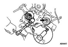
2. INSTALL NO.1 IDLER PULLEY AND NO.2 IDLER PULLEY a Apply adhesive 2 or 3 threads of the pivot bolt.
