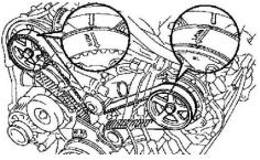
b Check that the timing marks of the camshaft timing pulleys and timing belt rear plates aligned. If not, turn the crankshaft 1 revolution (360 °).
