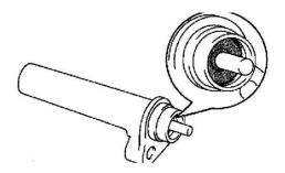
a Visually check the seal portion of the tensioner for oil leakage.
