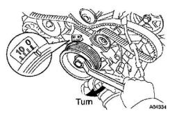
a Temporarily install the crankshaft pulley bolt. b Slowly turn the crankshaft pulley 2 revolutions from TDC to TDC. NOTICE: Always turn the crankshaft pulley clockwise.
