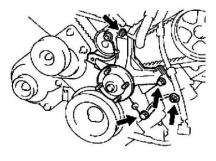
14. REMOVE FAN BRACKET Remove the 2 bolts, 2 nuts and fan bracket.
