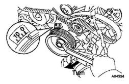
a Turn the crankshaft pulley and align its groove with timing mark "0" of the No.1 timing belt cover.
