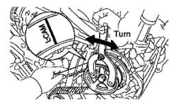
a Remove any oil or water on the LH camshaft timing pulley, and keep it clean.
