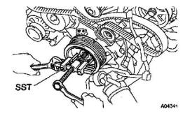
23. REMOVE CRANKSHAFT PULLEY Using SST, remove the crankshaft pulley. SST 09950-50012 (09951-05010, 09952-05010, 09953-05010, 09953-05020, 09954-05020)
