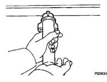
b Hold the tensioner with both hands and push the push rod strongly as shown to check that it doesn't move. If the push rod moves, replace the tensioner.
