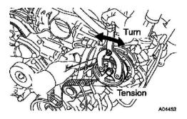
c Turn the LH camshaft timing pulley counterclockwise until there is tension between the crankshaft timing pulley and LH camshaft timing pulley.
