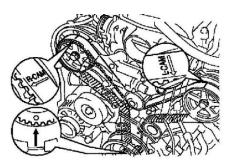
15. IF RE-USING TIMING BELT, CHECK INSTALLATION MARKS ON TIMING BELT Check that there are 3 installation marks on the timing belt by turning the crankshaft pulley as shown in the illustration.
