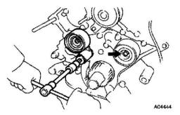
a Using a 10 mm hexagon wrench, remove the bolt, No.1 idler pulley and plate washer. b Remove the bolt and No.2 idler pulley.
