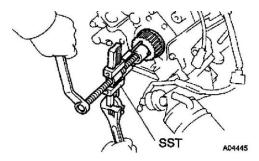
29. REMOVE CRANKSHAFT TIMING PULLEY Using SST, remove the timing pulley. SST 09950-50012 (09951-05010, 09952-05010, 09953-05010, 09953-05020, 09954-05010)
