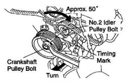
c Turn the crankshaft pulley approximately 50° clockwise, and put the timing mark of the crankshaft pulley in line with the centers of the crankshaft pulley bolt and the idler pulley bolt.
