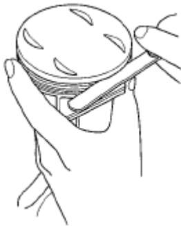
Fig. 47: Measuring Ring-To-Groove Clearance
