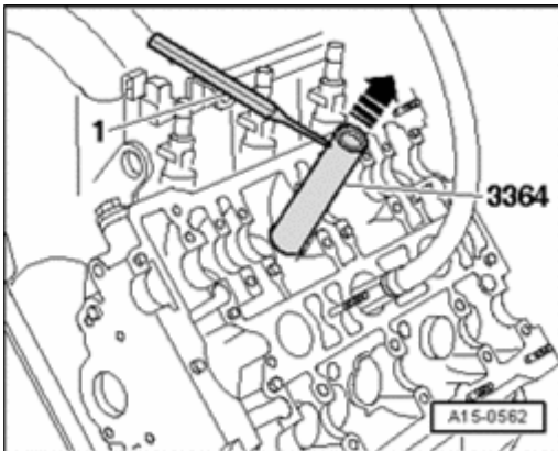
Fig. 215: Bringing Marking On Camshaft Gear To Alignment With Marking On Toothed Belt Guard Courtesy of VOLKSWAGEN UNITED STATES, INC.
