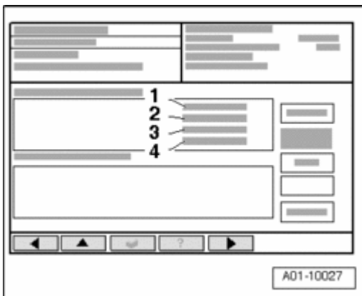
Fig. 6: Display On VAS 5051 - (Read-Out For Fuel Pressure In Fuel Rail) Courtesy of VOLKSWAGEN UNITED STATES, INC.
