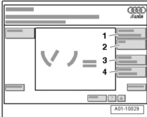
Fig. 2: Display On VAS 5051B - Vehicle Self-Diagnosis Button Courtesy of VOLKSWAGEN UNITED STATES, INC.
