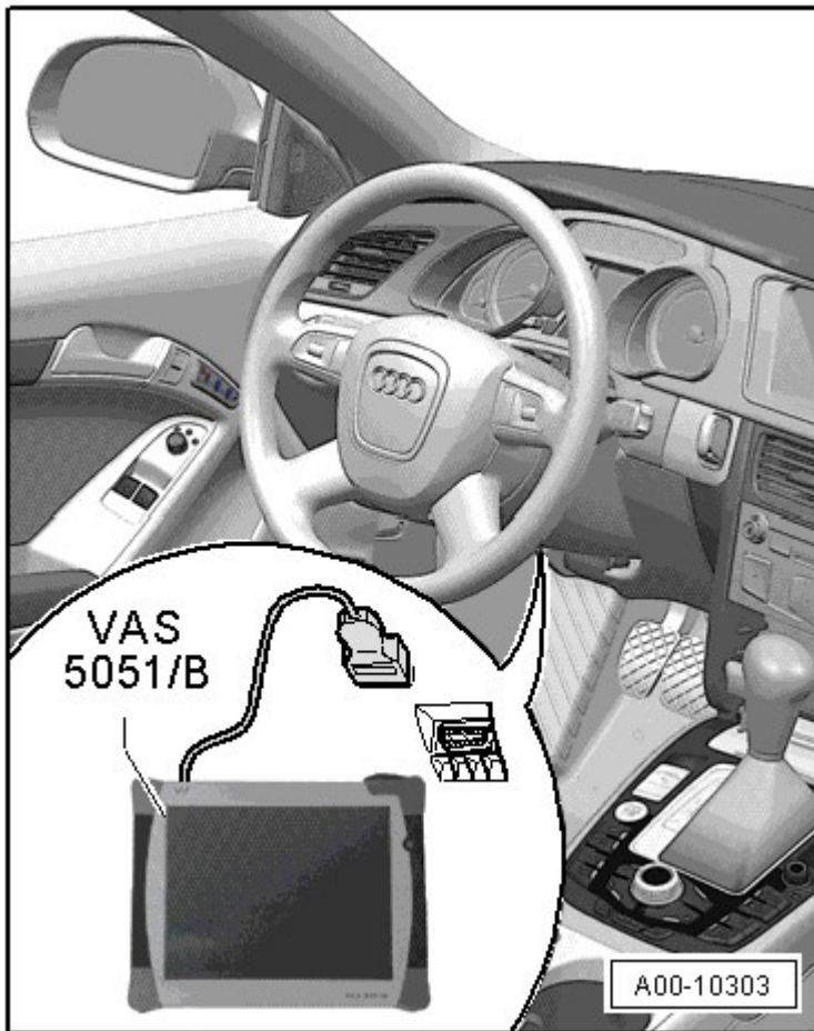
Fig. 1: Connecting Diagnostic Cable VAS 5051/5A To Diagnostic Connector Courtesy of AUDI OF AMERICA, LLC
