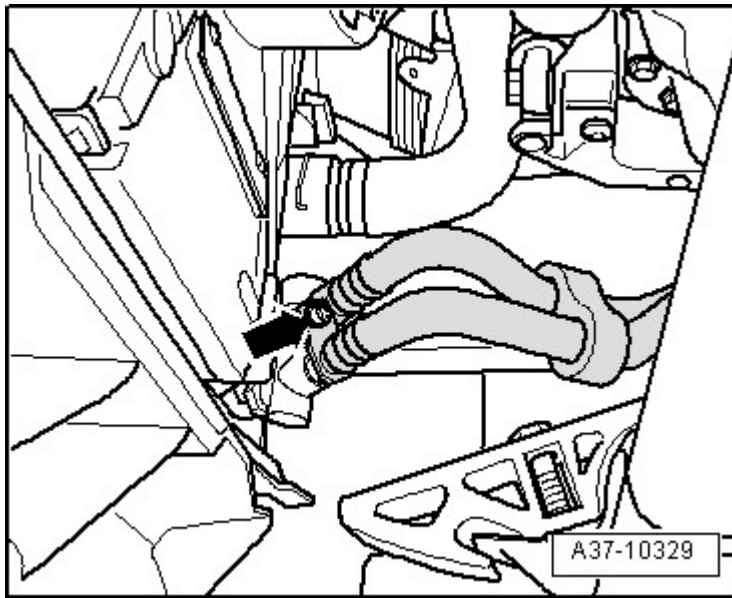
Fig. 141: Identifying Lines From Transmission Oil Cooler And Rear Mounting Bolts Courtesy of AUDI OF AMERICA, LLC
