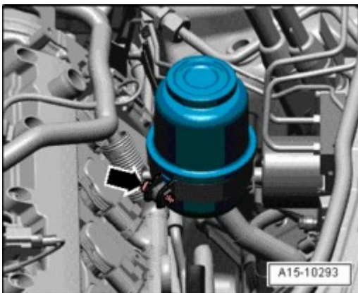
Fig. 327: Removing Bolt And Remove Power Steering Reservoir From Bracket, Hydraulic Lines Remain
