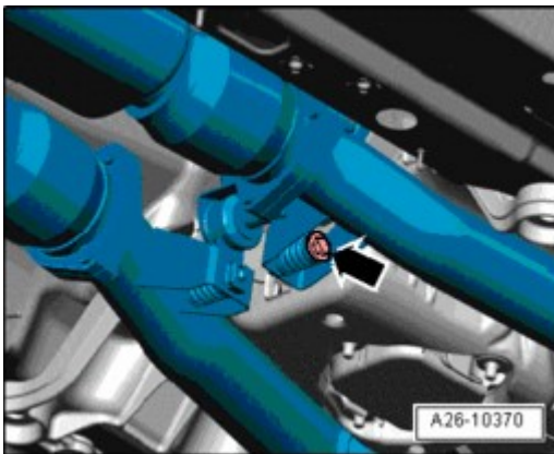
Fig. 102: Removing Bolt At Right Exhaust Tract Strap Courtesy of VOLKSWAGEN UNITED STATES, INC.
