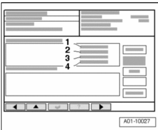
Fig. 12: Display On VAS 5051 - (Read-Out For Fuel Pressure In Fuel Rail) Courtesy of VOLKSWAGEN UNITED STATES, INC.
