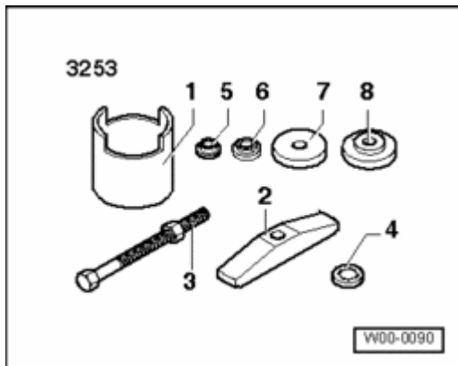
Fig. 153: Identifying Seal Installer 3253/6 From Assembly Tool 3253 Courtesy of VOLKSWAGEN UNITED STATES, INC.
