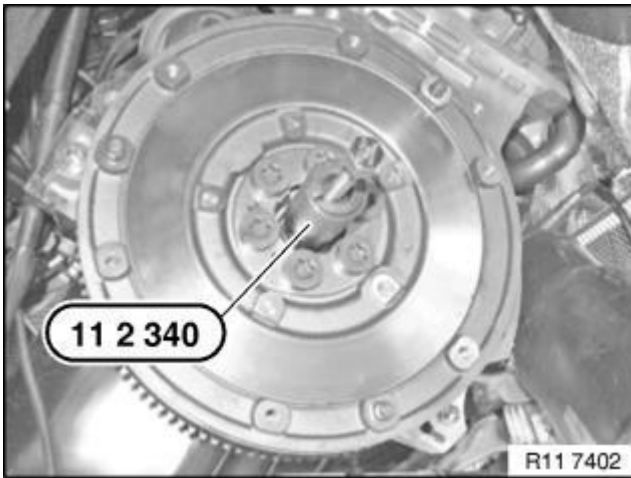
Fig. 133: Removing Guide Bearing With Special Tool 11 2 34 Courtesy of BMW OF NORTH AMERICA, INC.
