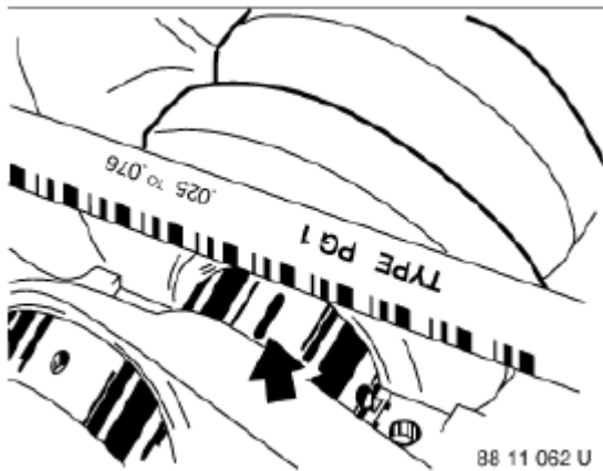
Fig. 132: Measuring Bearing Play Width Courtesy of BMW OF NORTH AMERICA, INC.
