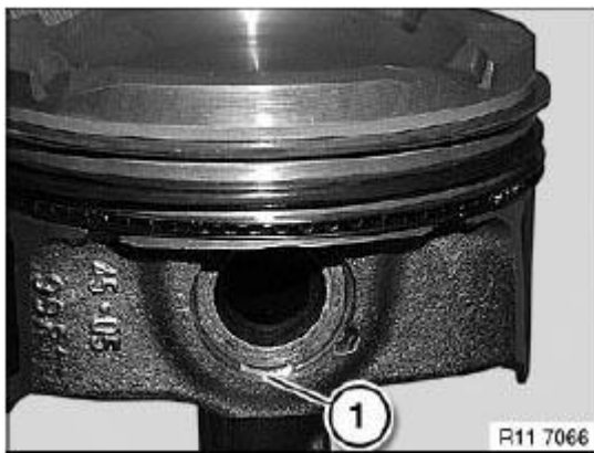
Fig. 211: Position Of Installing Piston Pin Circlip Courtesy of BMW OF NORTH AMERICA, INC.
