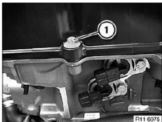
Fig. 47: Identifying Screws On Cylinder Head Cover
