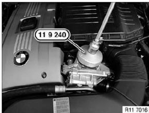
Fig. 6: Identifying Special Tool 11 9 240 For Releasing Oil Filter
