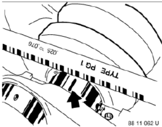
Fig. 137: Checking Bearing Play
