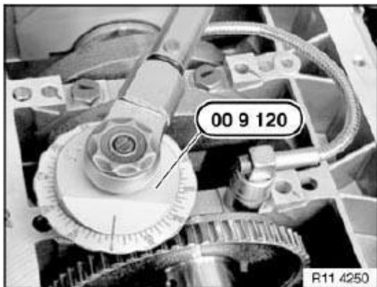
Fig. 122: Tightening Aluminum Screws Using 00 9 120 Courtesy of BMW OF NORTH AMERICA, INC.
