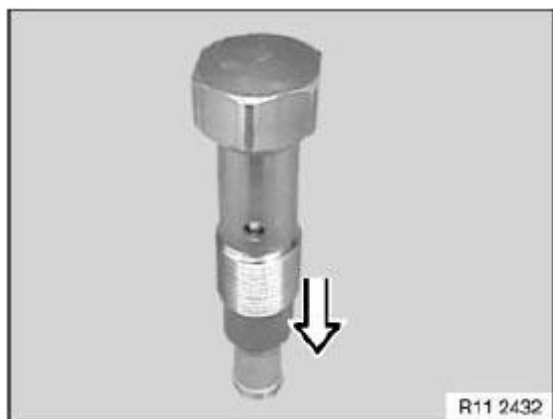
Fig. 292: Compressing Chain Tensioner Courtesy of BMW OF NORTH AMERICA, INC.
