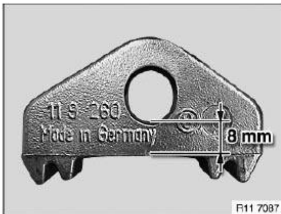
Fig. 186: Identifying Dimension Of Slot On Special Tool 11 9 260 Courtesy of BMW OF NORTH AMERICA, INC.
