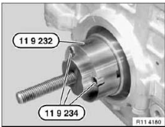
Fig. 129: Mounting Special Tool 11 9 232 With Screws To Crankshaft Courtesy of BMW OF NORTH AMERICA, INC.
