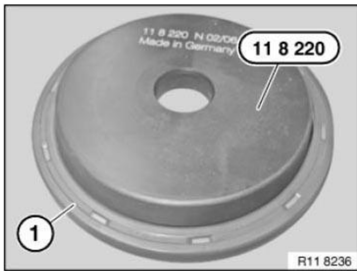
Fig. 186: Identifying Radial Shaft Seal On Special Tool 11 8 220 Courtesy of BMW OF NORTH AMERICA, INC.
