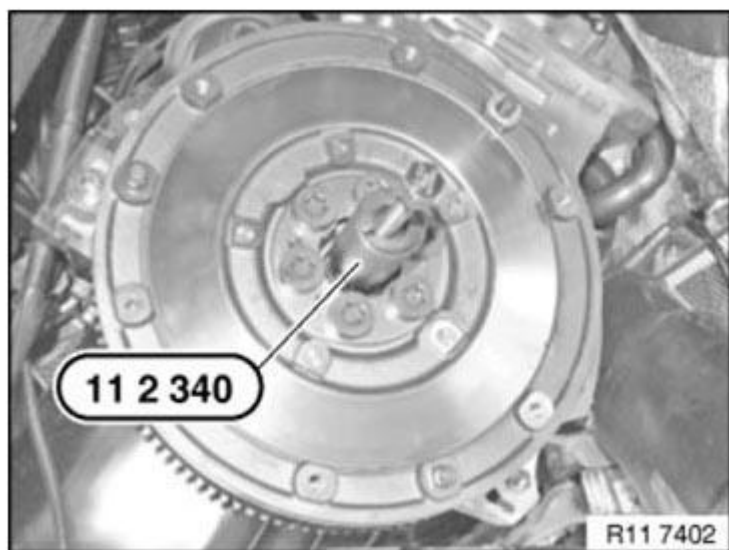
Fig. 325: Removing Guide Bearing Using Special Tool (11 2 340) Courtesy of BMW OF NORTH AMERICA, INC.
