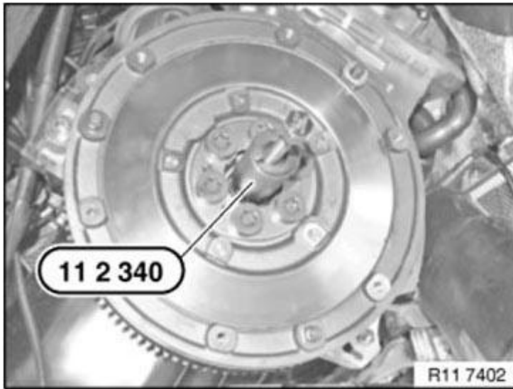
Fig. 139: Removing Guide Bearing Using Special Tool 11 2 340 Courtesy of BMW OF NORTH AMERICA, INC.
