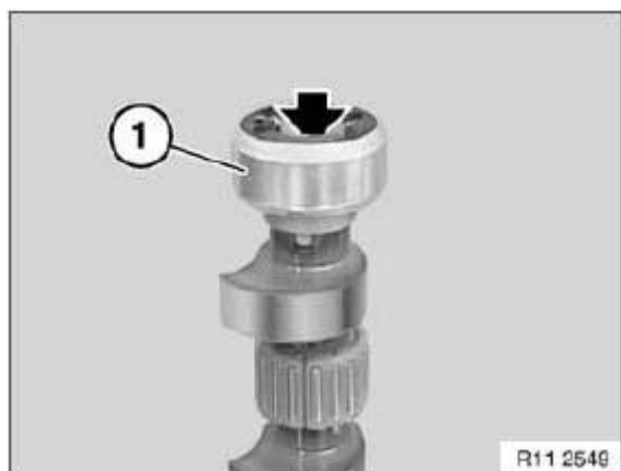
Fig. 301: Identifying Magnet Wheel
