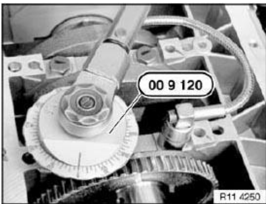
Fig. 133: Tightening Main Bearing Bolts Using Special Tool (00 9 120)
