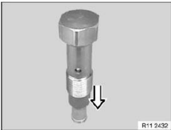
Fig. 246: Compressing Chain Tensioner Courtesy of BMW OF NORTH AMERICA, INC.
