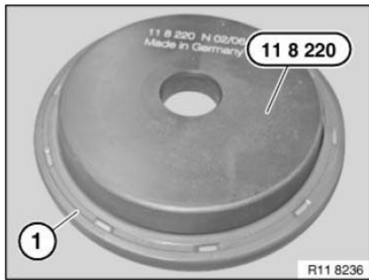
Fig. 101: Identifying Radial Shaft Seal On Special Tool 11 8 220 Courtesy of BMW OF NORTH AMERICA, INC.
