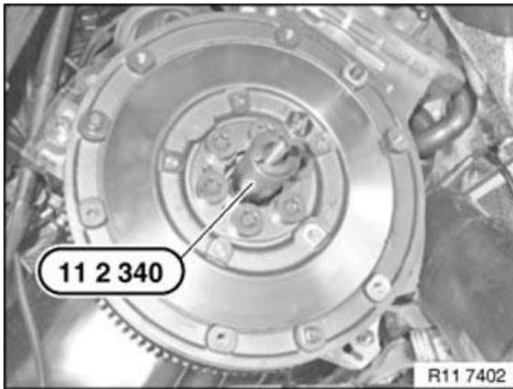
Fig. 129: Removing Guide Bearing Using Special Tool 11 2 340 Courtesy of BMW OF NORTH AMERICA, INC.
