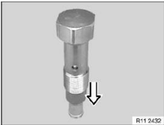
Fig. 259: Identifying Chain Tensioner Courtesy of BMW OF NORTH AMERICA, INC.
