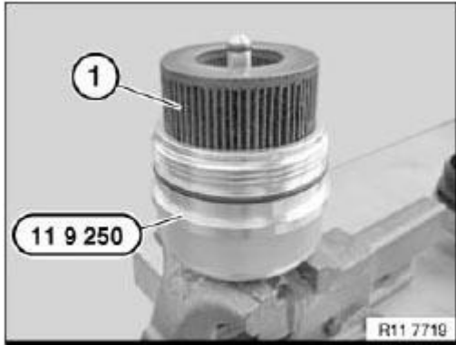
Fig. 344: Identifying Filter Element With Special Tool (11 9 250) Courtesy of BMW OF NORTH AMERICA, INC.
