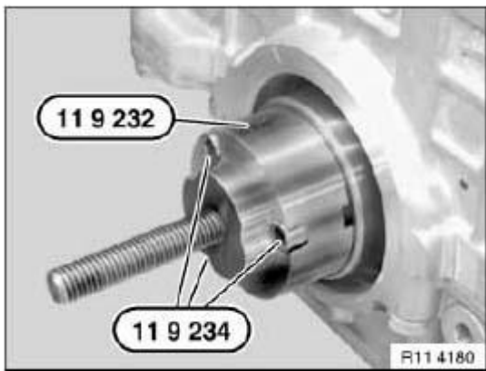
Fig. 71: Screwing Special Tool To Crankshaft Courtesy of BMW OF NORTH AMERICA, INC.
