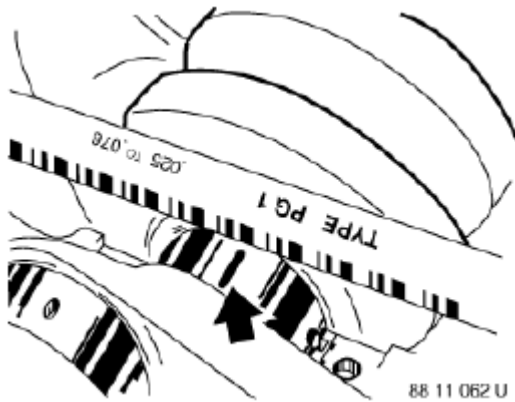
Fig. 128: Checking Bearing Play Using Plastic Gauge Courtesy of BMW OF NORTH AMERICA, INC.
