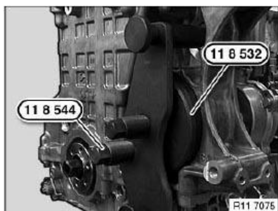
Fig. 80: Positioning Special Tool (11 8 532) On Sealing Cover Courtesy of BMW OF NORTH AMERICA, INC.
