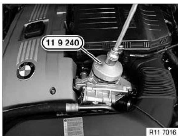
Fig. 4: Installing Oil Filter Cover Using Special Tool 11 9 240 Courtesy of BMW OF NORTH AMERICA, INC.
