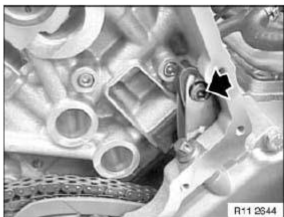
Fig. 73: Identifying Guide Rail Screw
