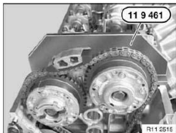
Fig. 361: Identifying Special Tool (11 9 461) Courtesy of BMW OF NORTH AMERICA, INC.
