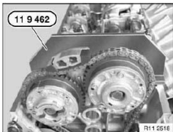
Fig. 466: Identifying Special Tool (11 9 462) Courtesy of BMW OF NORTH AMERICA, INC.
