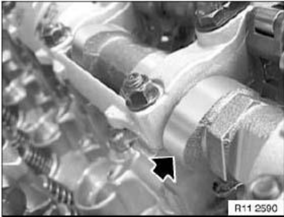
Fig. 387: Locating Inlet Camshaft Position Courtesy of BMW OF NORTH AMERICA, INC.
