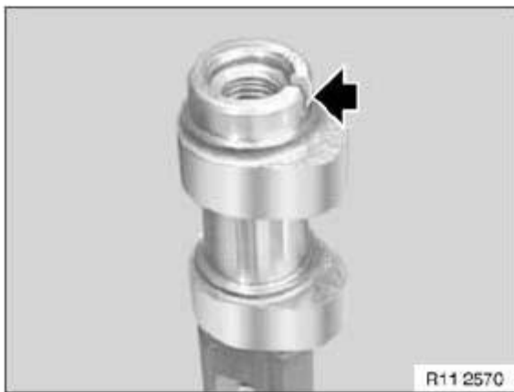
Fig. 295: Identifying Sensor Gear Lug Courtesy of BMW OF NORTH AMERICA, INC.
