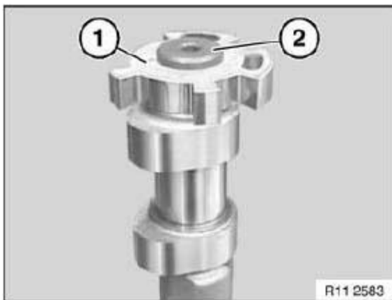
Fig. 317: Identifying Sensor Gear And Screw Courtesy of BMW OF NORTH AMERICA, INC.
