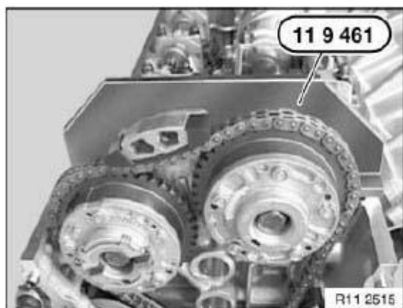
Fig. 351: Identifying Special Tool (11 9 461) On Inlet Camshaft Courtesy of BMW OF NORTH AMERICA, INC.
