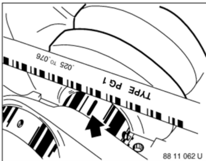
Fig. 151: Measuring Main Bearing Play Using Measurement Scale
