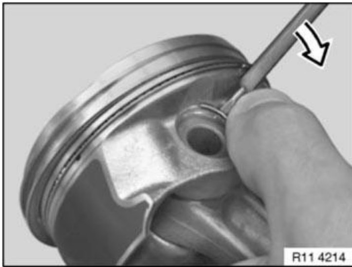
Fig. 192: Installing Retaining Ring Courtesy of BMW OF NORTH AMERICA, INC.
