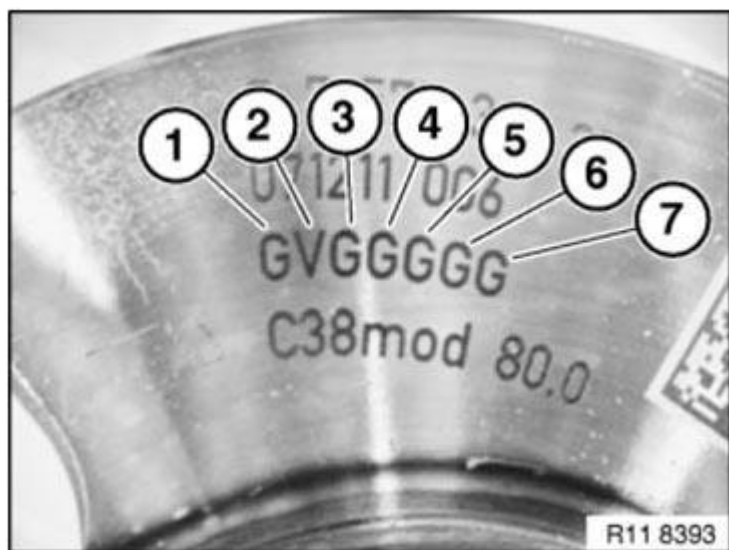
Fig. 143: Identifying Bearing Shell Classification For Relevant Bearing Position From 1 To 7 (Main Bearing Cap)
