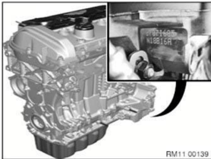
Fig. 18: Identifying Engine Identification Label (N12/N13/N14/N16/N18/W16) Courtesy of BMW OF NORTH AMERICA, INC.
