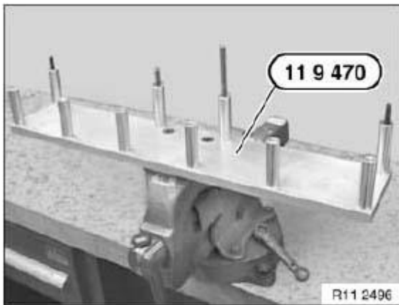
Fig. 532: Identifying Special Tool (11 9 470) Courtesy of BMW OF NORTH AMERICA, INC.
