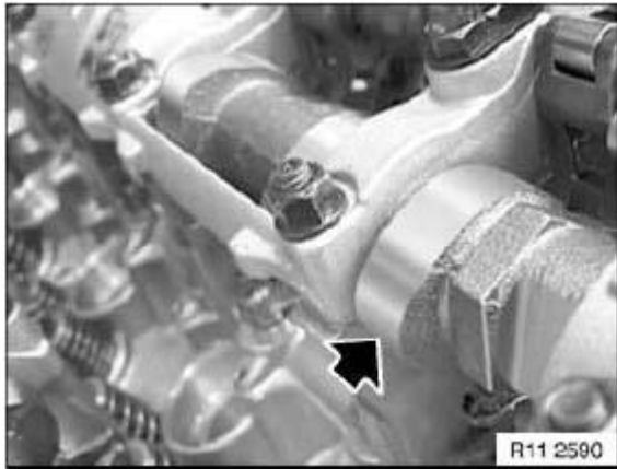
Fig. 391: Identifying Camshaft Lobe Courtesy of BMW OF NORTH AMERICA, INC.
