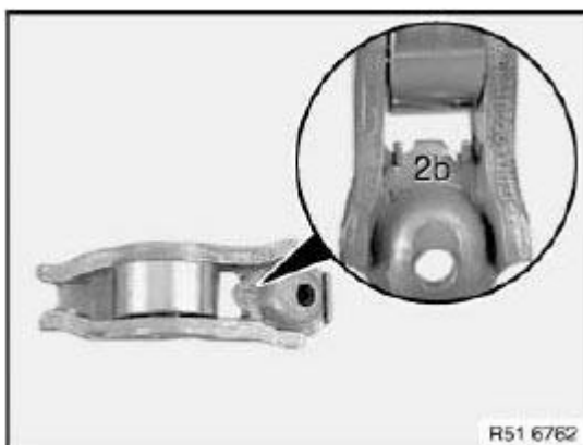
Fig. 570: Identifying Rocker Arms Tolerance Classes
