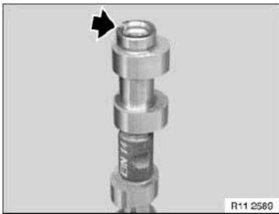
Fig. 364: Identifying Camshaft Groove Courtesy of BMW OF NORTH AMERICA, INC.
