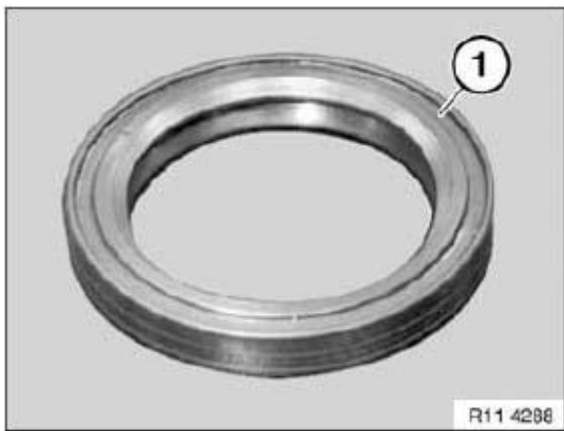
Fig. 44: Identifying Sealing Ring Courtesy of BMW OF NORTH AMERICA, INC.
