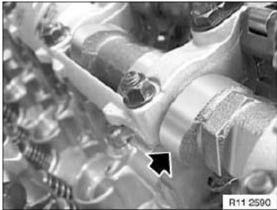
Fig. 343: Identifying Camshaft Lobe
