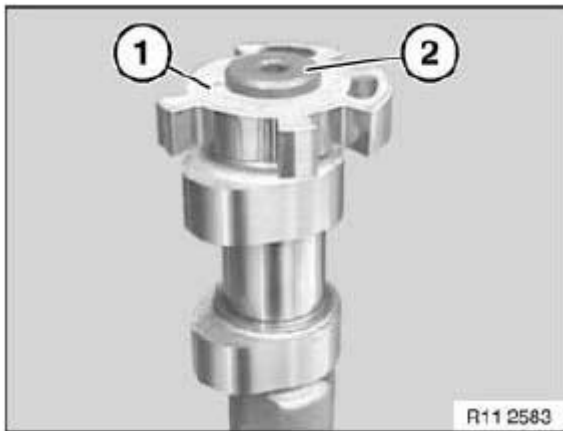
Fig. 473: Identifying Sensor Gear And Screw Courtesy of BMW OF NORTH AMERICA, INC.
