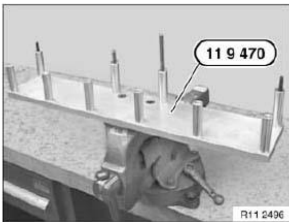
Fig. 718: Identifying Special Tool (11 9 470) Courtesy of BMW OF NORTH AMERICA, INC.
