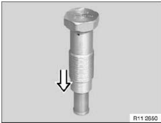
Fig. 97: Placing Chain Tensioning Piston On Level Surface Courtesy of BMW OF NORTH AMERICA, INC.
