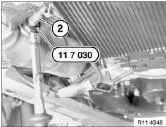
Fig. 1178: Identifying Monitor Sensor And Special Tool (11 7 030) Courtesy of BMW OF NORTH AMERICA, INC.
