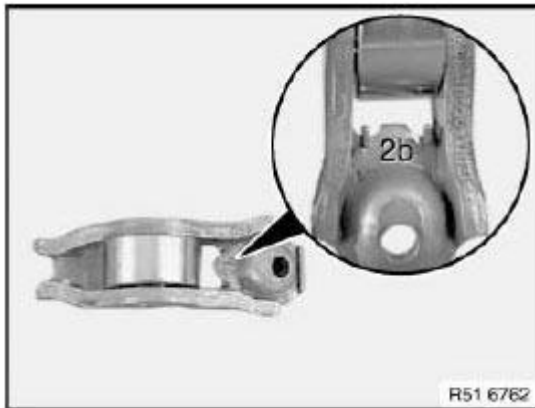
Fig. 537: Identifying Rocker Arms Tolerance Classes Courtesy of BMW OF NORTH AMERICA, INC.
