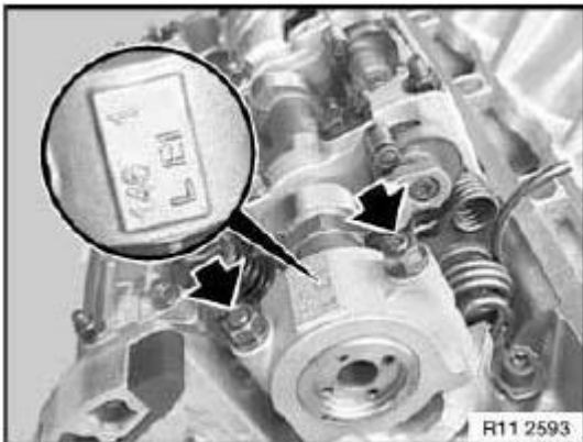
Fig. 1038: Identifying Bearing Cap L E1 And Nuts
