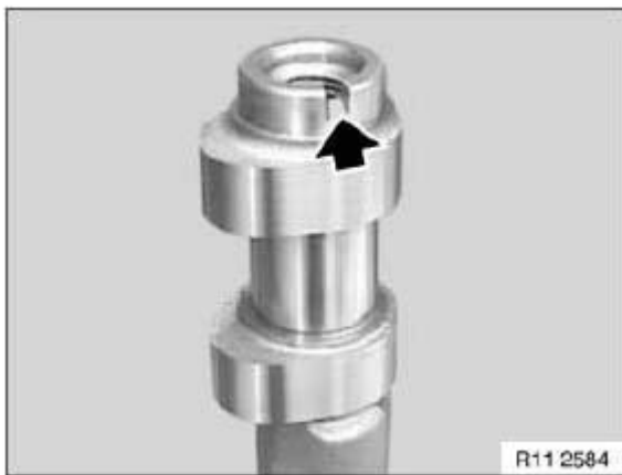
Fig. 472: Identifying Camshaft Groove Courtesy of BMW OF NORTH AMERICA, INC.
