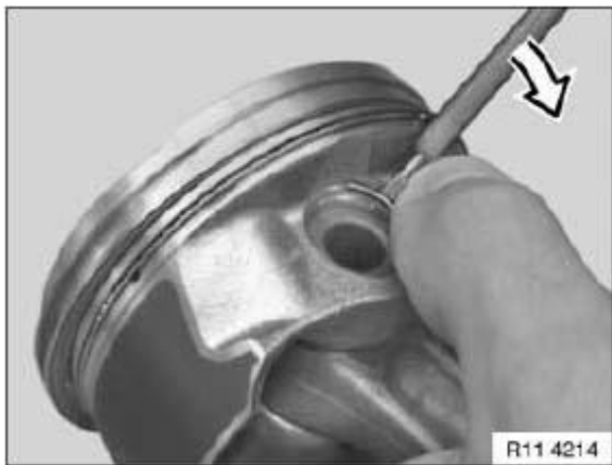
Fig. 218: Installing Retaining Ring Courtesy of BMW OF NORTH AMERICA, INC.
