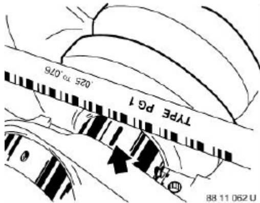
Fig. 190: Identifying Main Bearing Play In Measurement Scale Courtesy of BMW OF NORTH AMERICA, INC.
