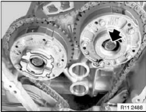
Fig. 873: Locating Screw On Inlet Adjustment Unit Courtesy of BMW OF NORTH AMERICA, INC.
