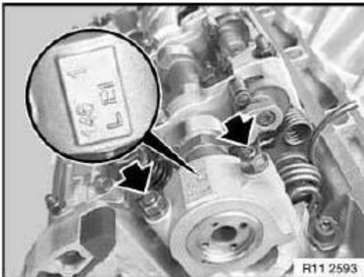
Fig. 658: Identifying Bearing Cap L E1 And Nuts
