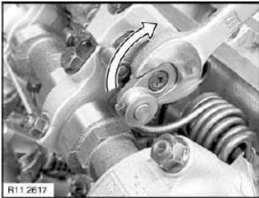
Fig. 593: Rotating Eccentric Shaft
