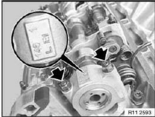
Fig. 777: Identifying Bearing Cap L E1 And Nuts Courtesy of BMW OF NORTH AMERICA, INC.
