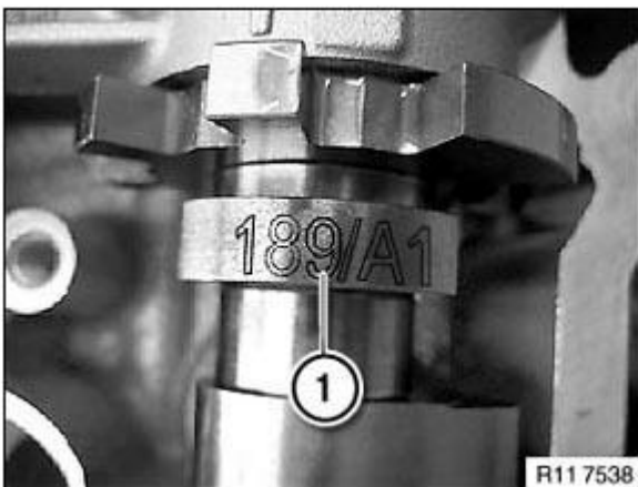
Fig. 200: Identifying Exhaust Camshaft Designation Courtesy of BMW OF NORTH AMERICA, INC.
