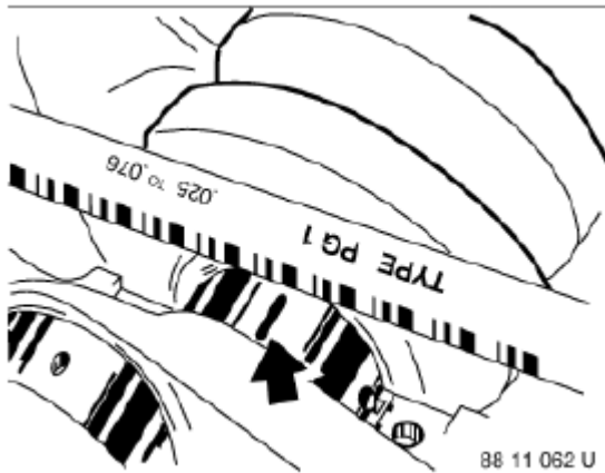
Fig. 96: Reading Bearing Play At Width Of Flattened Plastic Thread Courtesy of BMW OF NORTH AMERICA, INC.
