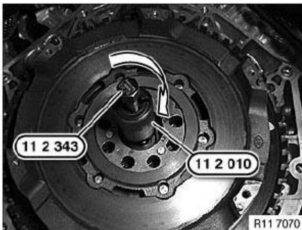
Fig. 143: Removing Roller Bearing Using Special Tool (11 2 343)
