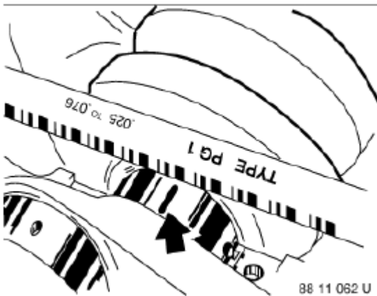
Fig. 120: Laying Plastic Thread (Plastigage) On Crankshaft
