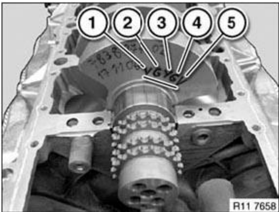
Fig. 125: Identifying Color Allocation On Crankshaft Courtesy of BMW OF NORTH AMERICA, INC.
