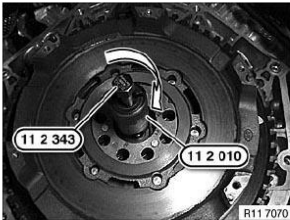
Fig. 133: Twisting Out Roller Bearing With Special Tool (11 2 343) Courtesy of BMW OF NORTH AMERICA, INC.
