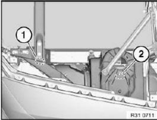
Fig. 43: Positioning Transverse Member With 2nd Person Helping On Designated Areas
