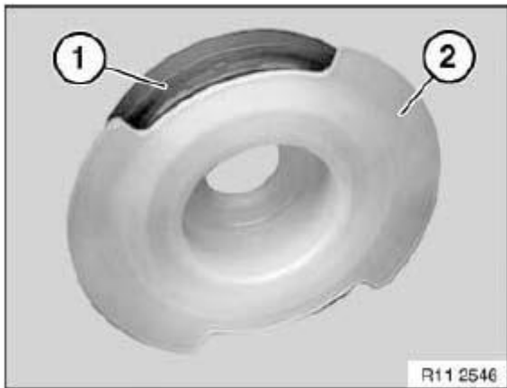
Fig. 113: Identifying Radial Shaft Seal With Support Sleeve Courtesy of BMW OF NORTH AMERICA, INC.
