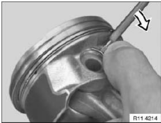
Fig. 181: Installing Retaining Ring Courtesy of BMW OF NORTH AMERICA, INC.
