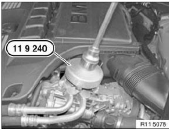
Fig. 382: Releasing Oil Filter Cap Using Special Tool 11 9 240 Courtesy of BMW OF NORTH AMERICA, INC.
