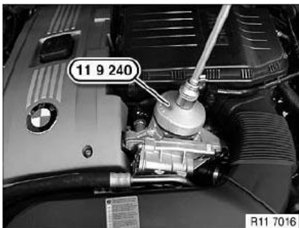
Fig. 22: Removing Oil Filter Cover Using Special Tool 11 9 240 Courtesy of BMW OF NORTH AMERICA, INC.
