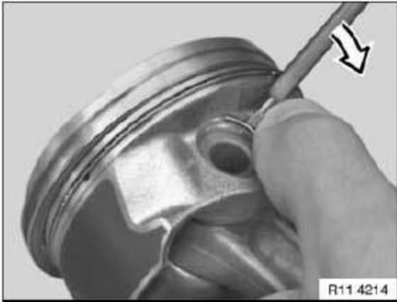
Fig. 208: Removing Piston Pin Circlip Courtesy of BMW OF NORTH AMERICA, INC.
