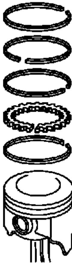
Fig. 366: Exploded View Of Piston Rings Courtesy of GENERAL MOTORS CORP.
