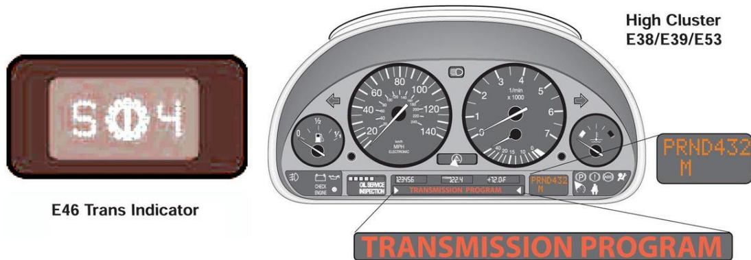
Fig. 24: Identifying Instrument Cluster Transmission Information Courtesy of BMW OF NORTH AMERICA, INC.
