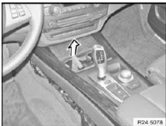
Fig. 147: Pulling Out Release Tool Courtesy of BMW OF NORTH AMERICA, INC.
