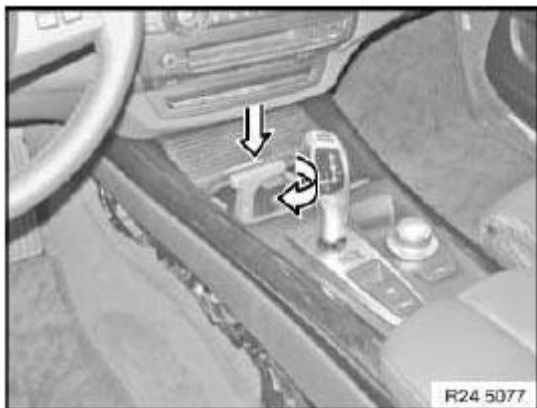
Fig. 146: Releasing Transmission Lock Courtesy of BMW OF NORTH AMERICA, INC.
