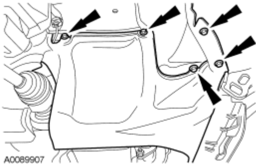
Fig. 742: Right Splash Shield Bolts Courtesy of FORD MOTOR CO.
