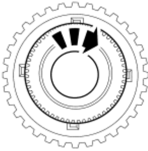
Fig. 398: Checking Forward One-Way Clutch Operation Courtesy of FORD MOTOR CO.
