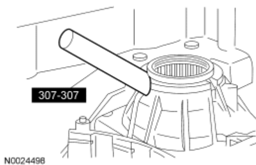
Fig. 521: Installing Final Drive Lube Tube Into Case Using Special Tools Courtesy of FORD MOTOR CO.
