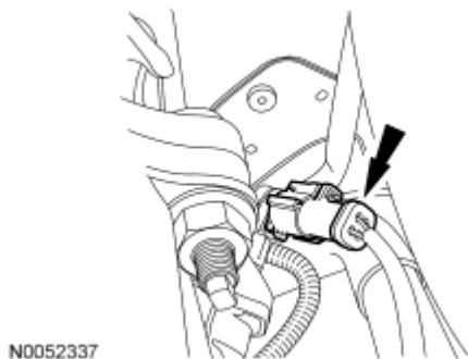
Fig. 467: Identifying RH Catalyst Monitor Electrical Connector Courtesy of FORD MOTOR CO.
