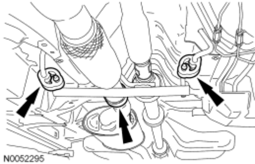
Fig. 456: Locating Exhaust Flexible Pipe Clamp & Exhaust Hangers Courtesy of FORD MOTOR CO.
