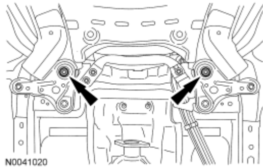
Fig. 504: Locating Rear Subframe Nuts Courtesy of FORD MOTOR CO.
