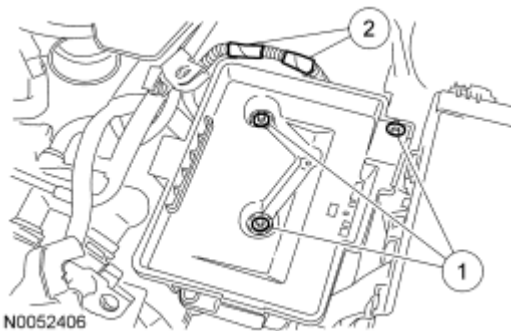
Fig. 542: Identifying Wiring Harness Fasteners, Battery Tray & Bolts Courtesy of FORD MOTOR CO.
