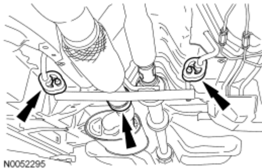
Fig. 249: Locating Exhaust Flexible Pipe Clamp & Exhaust Hangers Courtesy of FORD MOTOR CO.
