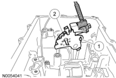
Fig. 219: Identifying TR Sensor In Transaxle Case Courtesy of FORD MOTOR CO.
