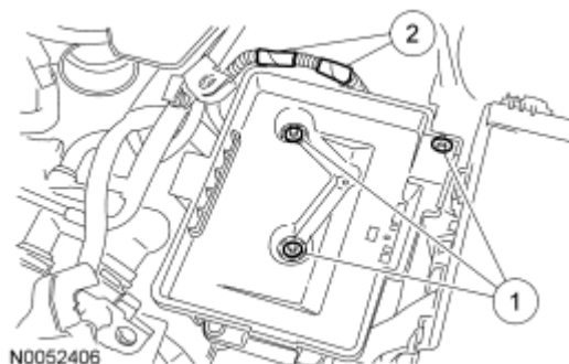
Fig. 273: Identifying Wiring Harness Fasteners, Battery Tray & Bolts Courtesy of FORD MOTOR CO.
