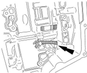
Fig. 107: Routing TSS Sensor Wiring Harness Through Cover & Transaxle Case Courtesy of FORD MOTOR CO.
