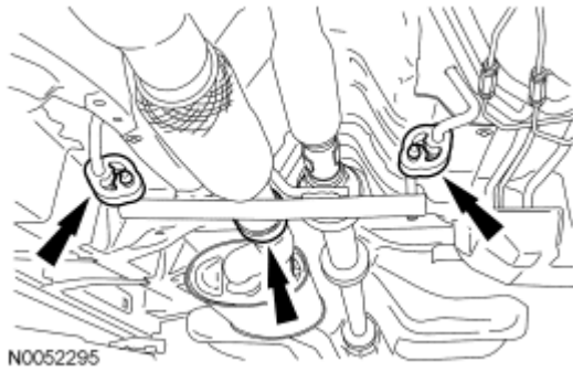
Fig. 512: Locating Exhaust Flexible Pipe Clamp & Exhaust Hangers Courtesy of FORD MOTOR CO.
