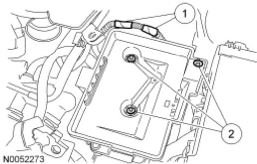
Fig. 260: Identifying Wiring Harness Fasteners, Battery Tray & Bolts Courtesy of FORD MOTOR CO.
