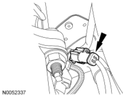
Fig. 498: Identifying RH Catalyst Monitor Electrical Connector Courtesy of FORD MOTOR CO.
