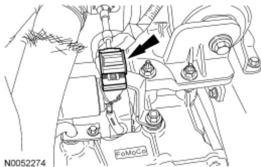
Fig. 379: Locating Selector Lever Cable End From Manual Lever Courtesy of FORD MOTOR CO.
