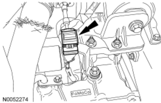
Fig. 417: Locating Selector Lever Cable End From Manual Lever Courtesy of FORD MOTOR CO.
