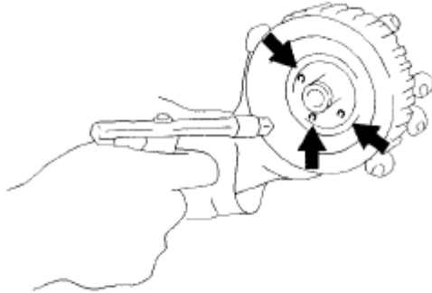
Fig. 82: Applying Compressed Air Through Fluid Passage Of 3-4 Clutch Drum Courtesy of MAZDA MOTORS CORP.
