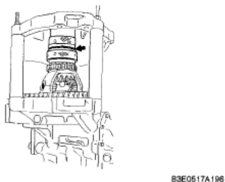
Fig. 231: Removing Converter Housing
