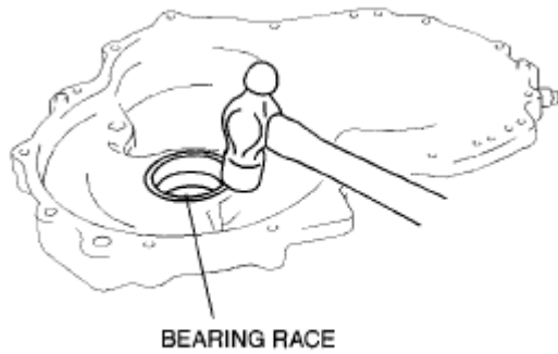
Fig. 222: Installing Bearing Race Into Transaxle Case Courtesy of MAZDA MOTORS CORP.
