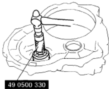
Fig. 232: Installing Bearing Race Into Converter Housing
