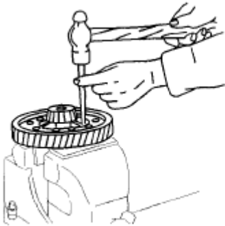
Fig. 210: Inserting Punch Into Roll Pin Hole Courtesy of MAZDA MOTORS CORP.
