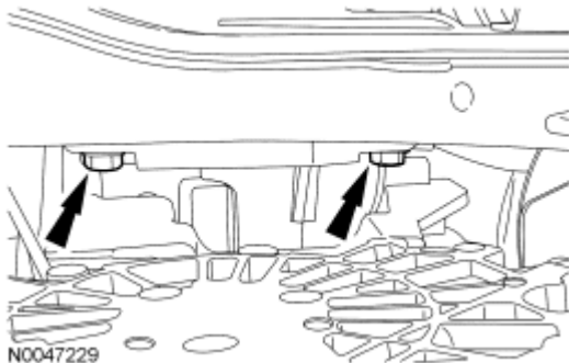
Fig. 200: Locating Rear Transaxle Insulator Bolts Courtesy of FORD MOTOR CO.
