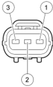
Fig. 26: Intermediate Shaft Speed Sensor Vehicle Harness C1088 Courtesy of FORD MOTOR CO.
