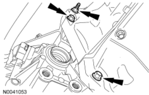
Fig. 254: Locating Back Torque Converter Housing Bolts Courtesy of FORD MOTOR CO.
