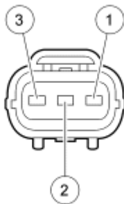
Fig. 25: Output Shaft Speed (OSS) Sensor Vehicle Harness C193 Courtesy of FORD MOTOR CO.
