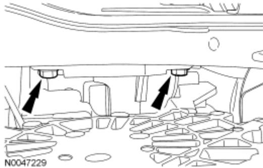
Fig. 201: Locating Rear Transaxle Insulator Bolts Courtesy of FORD MOTOR CO.
