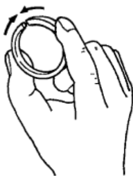
Fig. 77: Squeezing Seal Ring Courtesy of HYUNDAI MOTOR CO.
