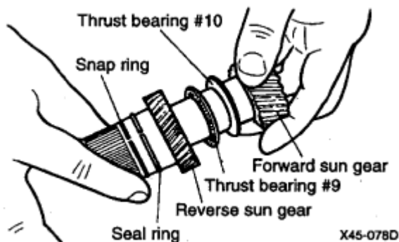
Fig. 78: Assembling Reverse Sun Gear & Forward Sun Gear Courtesy of HYUNDAI MOTOR CO.
