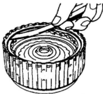
Fig. 176: Checking Clearance Between Snap Ring & Clutch Reaction Plate Courtesy of HYUNDAI MOTOR CO.
