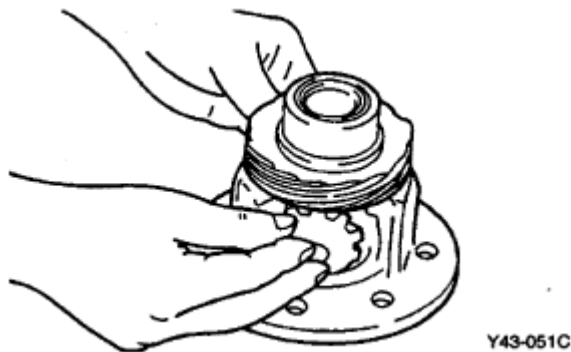
Fig. 197: Removing/Installing Gear In Differential Case Courtesy of HYUNDAI MOTOR CO.
