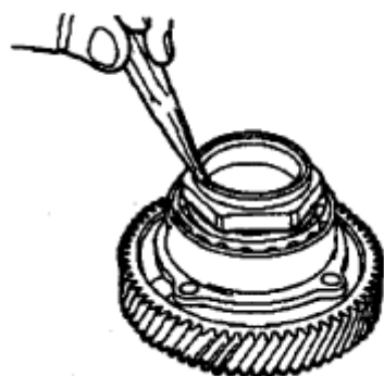
Fig. 192: Caulking Lock Nut Courtesy of HYUNDAI MOTOR CO.
