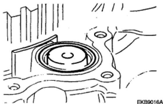
Fig. 109: Installing Direct Clutch, Accumulator Spring, Piston, & O-Ring Courtesy of HYUNDAI MOTOR CO.
