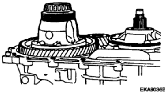
Fig. 81: Measuring End Play When Applying 49N(5Kgf,11lbf) Weight And 245.17kPa(2.5 Bar, 35.56psi) Air Pressure On Plates And Discs Courtesy of KIA MOTORS AMERICA, INC.
