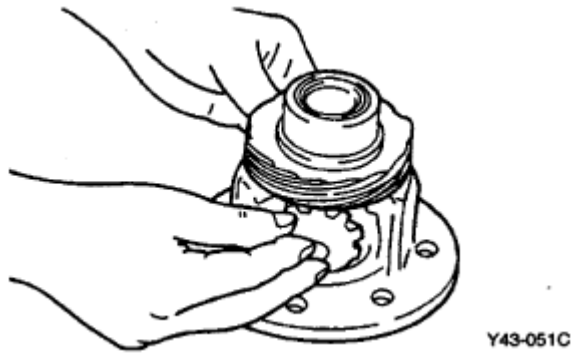
Fig. 145: Applying Liquid Gasket With 0.102in (2.6mm) Thickness Courtesy of KIA MOTORS AMERICA, INC.
