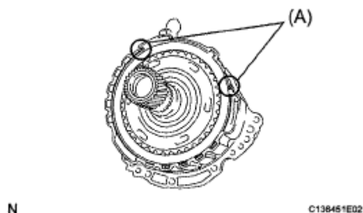
Fig. 442: Identifying Snap Ring
