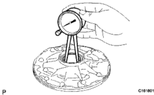
Fig. 657: Measuring Inside Diameter Of Oil Pump Body Bush Courtesy of TOYOTA MOTOR SALES, U.S.A., INC.
