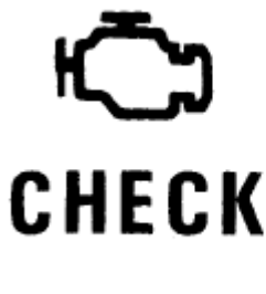
Fig. 17: Identifying Malfunction Indicator Lamp
