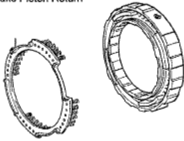
Fig. 496: Installing 2nd Brake Piston Return Spring Courtesy of TOYOTA MOTOR SALES, U.S.A., INC.
