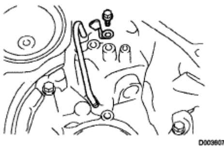
Fig. 337: Installing Differential Gear Lube Apply Tube
