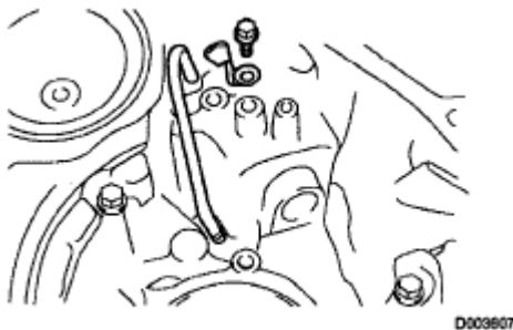
Fig. 347: Installing Differential Gear Lube Apply Tube Courtesy of TOYOTA MOTOR SALES, U.S.A., INC.
