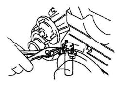
(c) Remove the 1.5 mm hexagon wrench from the tensioner.
