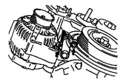
(a) Temporarily install the tensioner with the 2 bolts. (b) Alternately tighten the 2 bolts.
