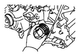
(a) Align the pulley set key with the key groove of the pulley. (b) Slide on the timing pulley facing the flange side inward.
