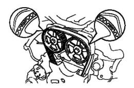
HINT (When re-using timing belt): Align the match-marks of the timing belt and camshaft timing pulleys.
