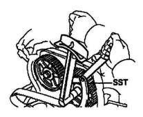
(c) Using SST, tighten the pulley bolt. SST 09960-10010 (09962-01000. 09963-01000)
