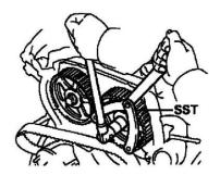
9. REMOVE CAMSHAFT TIMING PULLEYS
