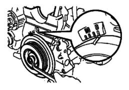
(a) Turn the crankshaft pulley, and align its groove with timing mark "0" of the No.1 timing belt cover.
