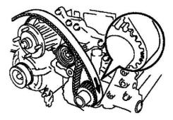
(c) Install the timing belt on the crankshaft timing pulley and idler pulley.
