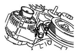
(a) Alternately loosen the 2 bolts, and remove them, the tensioner and dust boot.
