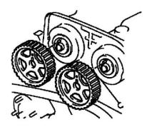
(a) Align the camshaft knock pin with the groove of the pulley, and slide on the timing pulley. (b) Temporarily in8tall the timing pulley bolt.
