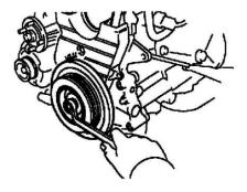
(a) Slowly turn the crankshaft pulley 2 revolutions from TDC to TDC.
