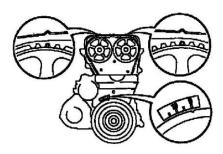
(b) Check that each pulley aligns with the timing marks as shown in the illustration. If the marks do not align, remove the timing belt and reinstall it.
