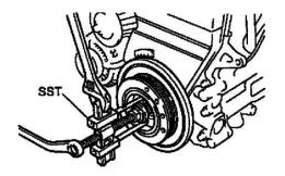
(c) Using SST, remove the pulley. SST 09950-50010 (09954-05030. 09551-05010, 09552-05010. 09553-05020)
