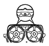
(b) Check that the timing marks of the camshaft timing pulleys are aligned with the timing marks of the No.4 timing belt cover. If not, turn the crankshaft 1 revolution (380°).
