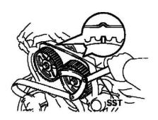
(b) Using SST. align the timing marks of the camshaft timing pulleys and No.4 timing belt cover. SST 09960-10010 (09962-01000.09963-01000)
