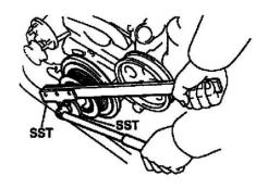
(a) Using SST, loosen the pulley bolt. SST 09213-70010,09330-00021 (b) Remove the pulley bolt.
