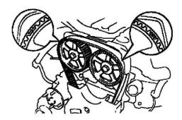
HINT (Re-using timing belt): Place matchmarks on the timing belt and camshaft timing pulleys as shown in the illustration.
