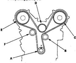
9. Install the timing belt in a counterclockwise sequence starting with the drive pulley.
