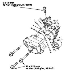
8. Install the engine mount bracket.
