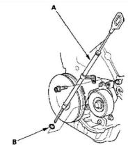
9. Remove the dipstick and tube (A); discard the O-ring (B).
