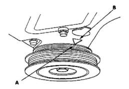
17. Turn the crankshaft pulley so its white mark (A) lines up with the pointer (B).
