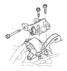
8. Remove the side engine mount bracket.
