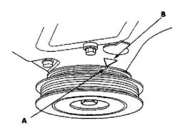
1. Turn the crankshaft so its white mark (A), lines up with the pointer (B).
