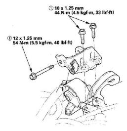
18. Install the side engine mount bracket, then tighten the mounting bolts in the numbered sequence.
