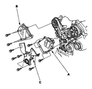
12. Remove the front upper cover (A), rear upper cover (B), and lower cover (C).
