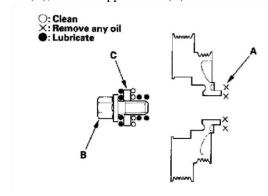
14. Clean all oil off the inside face (A) of the crankshaft pulley, and apply lubricant to the pulley bolt (B) and washer (C).
