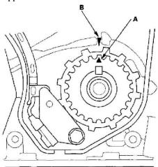
2. Set the timing belt drive pulley to TDC by aligning the TDC mark (A) on the tooth of the timing belt drive pulley with the pointer (B) on the oil pump.
