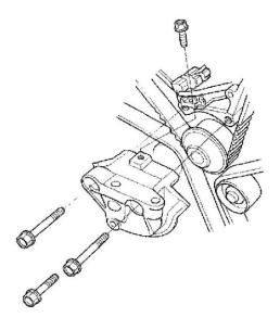
15. Remove the engine mount bracket.
