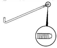
13. Remove one of the battery clamp bolts from the battery tray, and grind the end of it.
