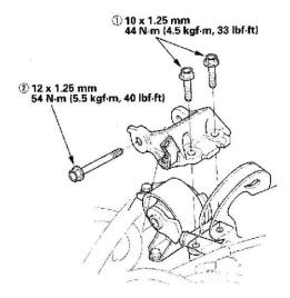
22. Install the side engine mount bracket, then tighten the mounting bolts in the numbered sequence.
