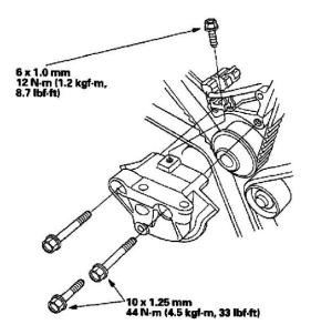
12. Install the engine mount bracket.
