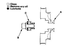
10. Clean any oil off the inside face (A) of the crankshaft pulley, and apply lubricant to the pulley bolt (B) and washer (C).
