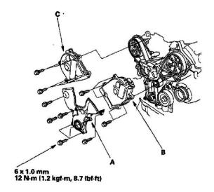
9. Install the lower cover (A), front upper cover (B), and rear upper cover (C).
