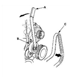
5. Use the belt tension release arm (A) to move the auto-tensioner (B), then remove the alternator belt (C).
