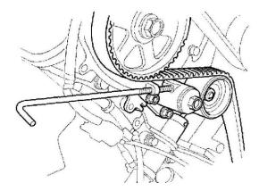
14. Screw the battery clamp bolt in to hold the timing belt adjuster in its current position. Tighten it by hand, do not use a wrench.
