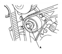
16. Loosen the idler pulley bolt (A) about five or six turns, then remove the timing belt.
