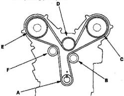
5. Install the timing belt in a counterclockwise sequence starting with the drive pulley. Take care not to damage the timing belt when installing it.
