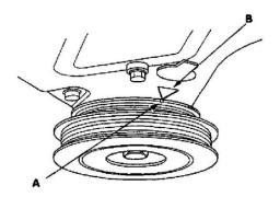
13. Turn the crankshaft pulley so its white mark (A) lines up with the pointer (B).
