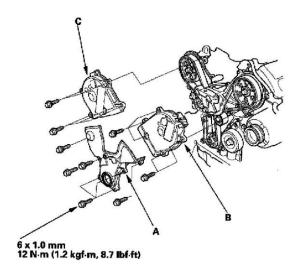
13. Install the lower cover (A), front upper cover (B), and rear upper cover (C).
