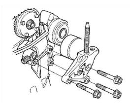
13. Remove the side engine mount bracket.
