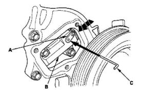
3. Align the holes on the lock (A) and the auto-tensioner (B), then insert a 1.5 mm (0.06 inch) diameter pin (C) into the holes. Turn the crankshaft clockwise to secure the pin.
