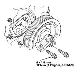
Timing Chain Tensioner Torque
