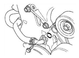
8. Remove the oil cooler hose joint pipe from the water pump (K20A2 engine).
