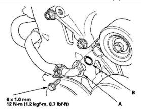
21. Install the oil cooler hose joint (A), using a new O-ring (B) (K20A2 engine).
