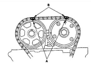
4. Install the cam chain on the VTC actuator and exhaust camshaft sprocket with the punch marks (A) aligned with the two colored pieces (B).
