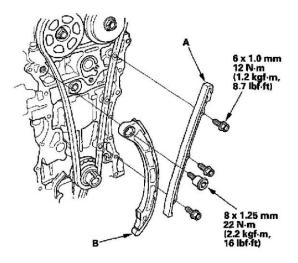
5. Install the cam chain guide A (A) and tensioner arm (B).
