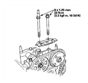
7. Install the cam chain guide B.
