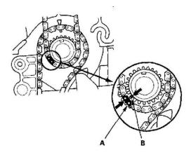
3. Install the cam chain on the crankshaft sprocket with the colored piece (A) aligned with the punch mark (B) on the crankshaft sprocket.
