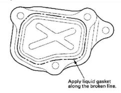
5. Apply liquid gasket, P/N 08718-0009, evenly to the chain case mating surface of the chain case cover and to the inner threads of the holes.
