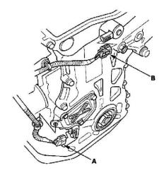
20. Connect the CKP sensor connector (A) and VTC oil control solenoid valve connector (B).
