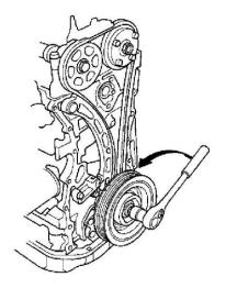
16. Turn the crankshaft counterclockwise to compress the auto-tensioner.
