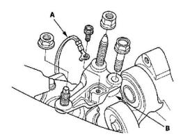
12. Remove the ground cable (A), and remove the upper bracket (B).
