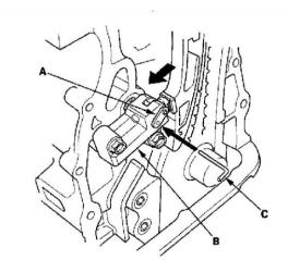
17. Align the holes on the lock (A) and the auto-tensioner (B), then insert a 1.5 mm (0.06 inch) diameter pin (C) into the holes. Turn the crankshaft clockwise to secure the pin.
