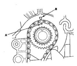
1. Set the crankshaft to TDC. Align the TDC mark (A) on the crankshaft sprocket with the pointer (B) on the cylinder block.
