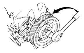
2. Turn the crankshaft counterclockwise to compress the auto-tensioner.
