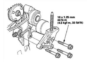
16. Install the side engine mount bracket.
