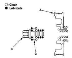
22. Clean the crankshaft pulley (A) and pulley bolt (B), and apply lubricant to the pulley bolt and washer (C).
