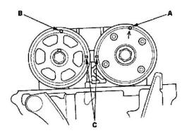
2. Set the camshafts to TDC. The punch mark (A) marked with an arrow on the Variable Valve Timing Control (VTC) actuator and the punch mark (B) on the exhaust camshaft sprocket should be at the top. Align the TDC marks (C) on the VTC actuator and exhaust camshaft sprocket.
