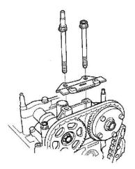
19. Remove the cam chain guide B.
