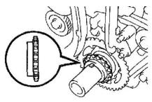
7. INSTALL CRANKSHAFT TIMING SPROCKET
