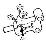
b. Inspect the oil jet (No.2 chain tensioner). Check the oil jet for damage or clogging.
