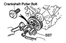
HINT: If necessary, remove the pulley with SST and crankshaft pulley bolt.
