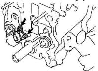
22. 3 RZ-FE: REMOVE NO.4 VIBRATION DAMPER Remove the 2 bolts and No.4 damper.
