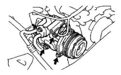
a. Remove the 4 bolts, and disconnect the compressor from the bracket.
