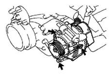
c. Remove the lock bolt, pivot bolt and generator.
