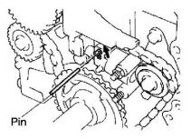
a. Install a pin to the No.2 chain tensioner and lock the plunger.
