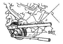
b. Using SST, install and torque the pulley bolt.
