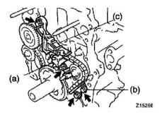
a. Install the No.2 chain tensioner with the nut.
