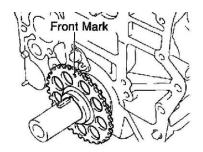
5. 2 RZ-FE: INSTALL CRANKSHAFT POSITION SENSOR ROTOR
