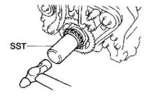
HINT: If necessary, install the sprocket with SST.
