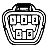
Fuel Sender Gauge Connector Front View:
