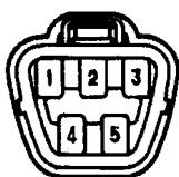
Fuel Sender Gauge Connector Front View:
