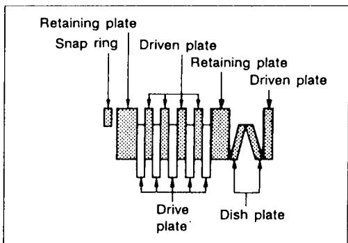
**Install drive plates, driven plates and retaining plate.**
