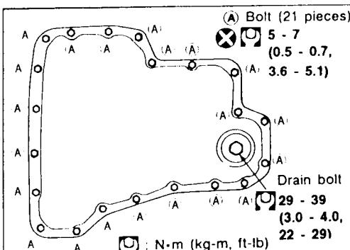
Remove oil pan and oil pan gasket.
