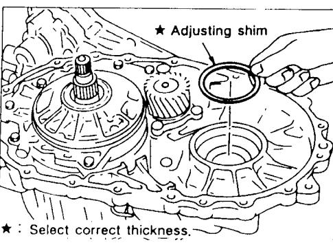
24 Remove differential side bearing adjusting shim from transmission case.
