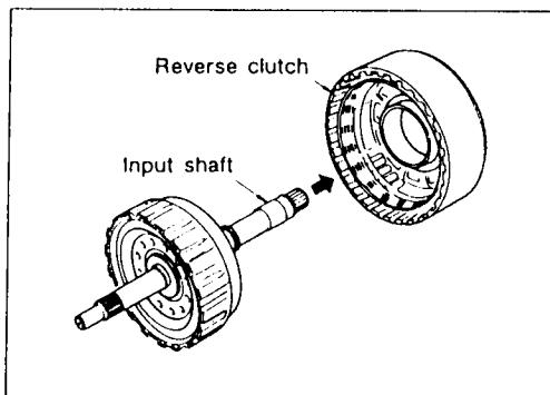
Remove input shaft assembly (high clutch) from reverse clutch.
