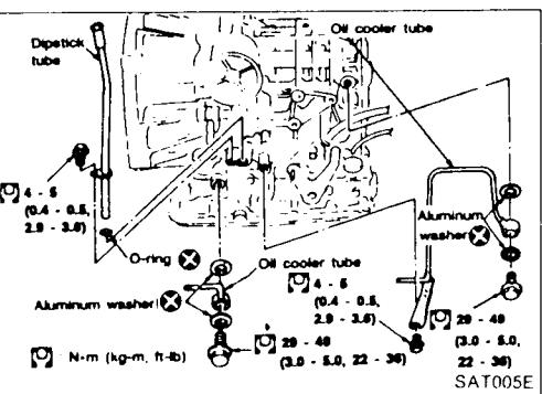
15. Install oil charging pipe and oil cooler tube to transmission case.
