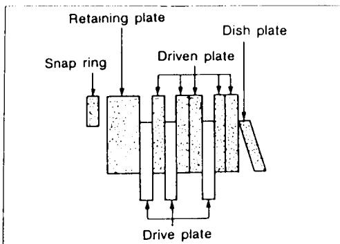
Install drive plates, driven plates, retaining plate and dish plate for overrun clutch.
