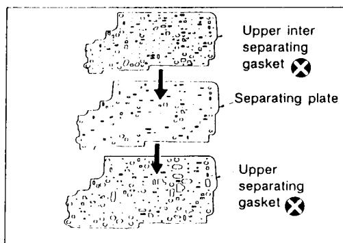
Install upper separating gasket, upper inter separating gasket and upper separating plate in order shown
