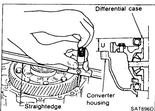
3. Place final drive assembly on converter housing.
