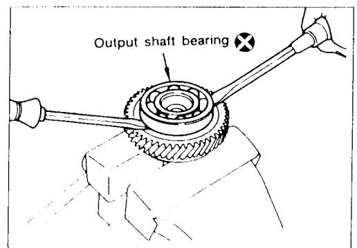
Remove output shaft bearing with screwdrivers.
