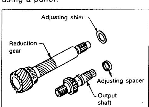
Remove reduction gear and output shaft.
