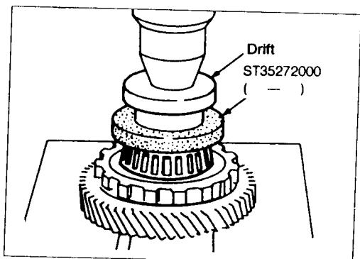
Press idler gear bearing inner race on idler gear.
