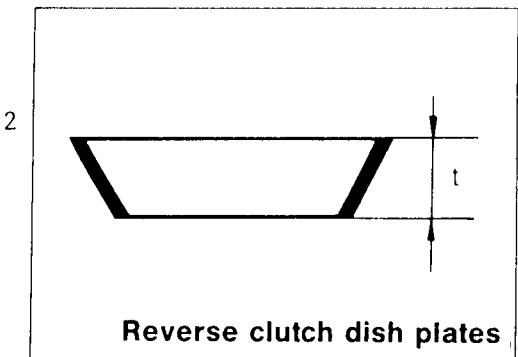
Check for deformation or damage.
