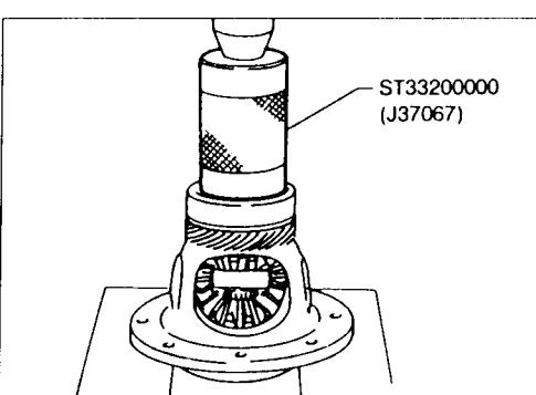
Press differential side bearings on differential case.
