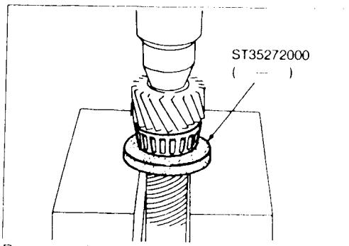
Press reduction gear bearing inner race on reduction gear.
