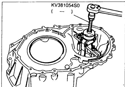
Remove differential side bearing outer race from converter housing (RL4F03V).
