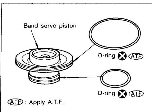
Install D-rings to servo piston retainer.
