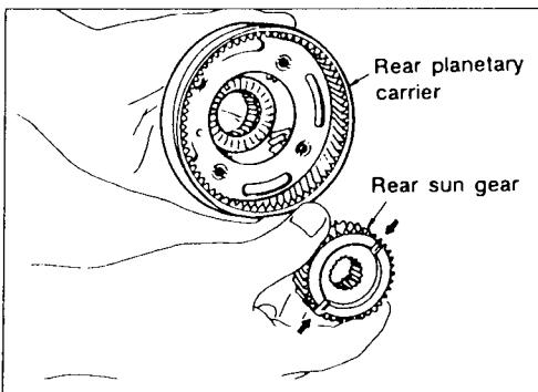
Remove rear sun gear from rear planetary carrier.
