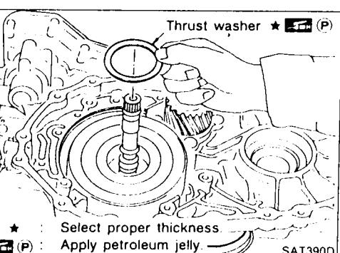
6. Place thrust washer selected in reverse clutch end play step on reverse clutch drum.
