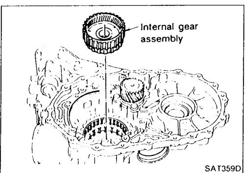
7. Install rear internal gear assembly.
