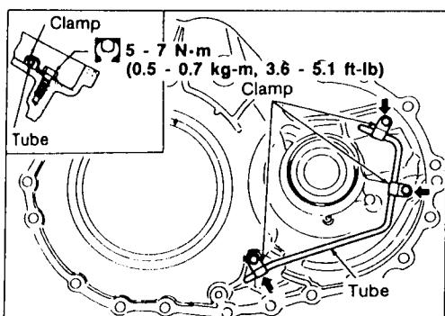
Remove oil tube from converter housing.
