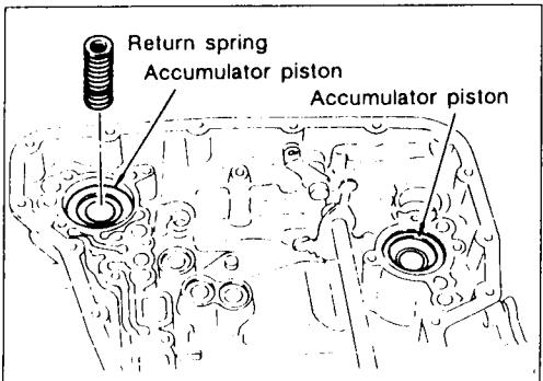
11 Remove return spring from 3-R accumulator piston.
