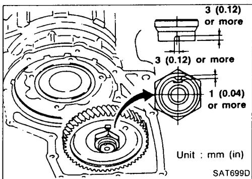
8. After properly adjusting turning torque, clinch idler gear lock nut as shown (only RL4F03V).
