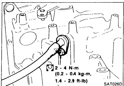
9. Install throttle wire to transmission case.
