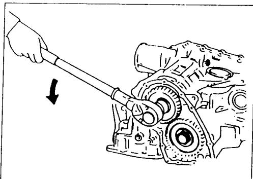
Remove idler gear and output gear lock nuts.
