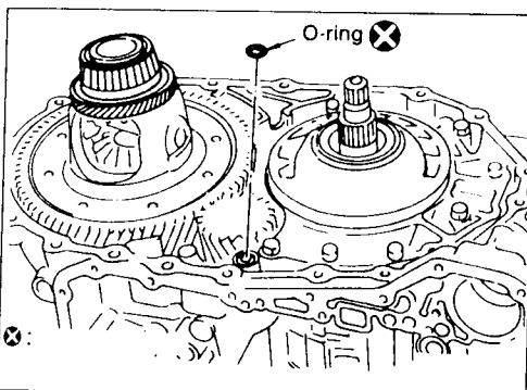
21 Remove O-ring from differential oil port.
