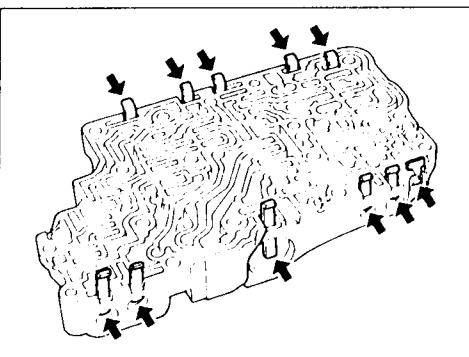
Check to see that retainer plates are properly positioned in upper body.
