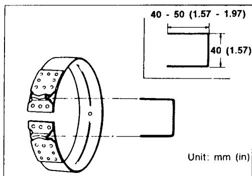
Check brake band facing for damage, cracks, wear or burns.
