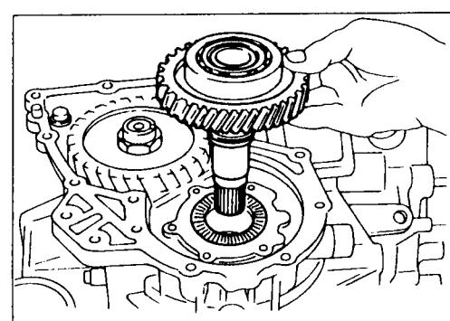
Remove output shaft assembly.
