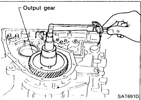
9. Measure turning torque of output shaft.
