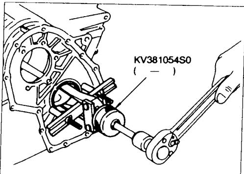
Remove idler gear bearing outer race from transmission case.
