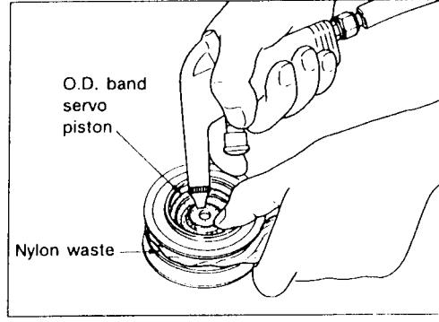
Apply compressed air to oil hole in O.D. servo piston retainer to remove O.D. band servo piston from retainer.
