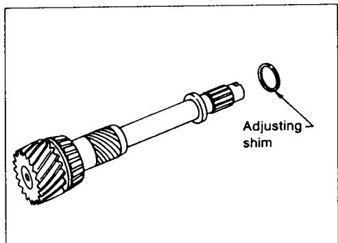
Remove adjusting shim from reduction gear.
