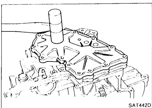
9. Install side cover on transmission case and tighten fixing bolt to the specified torque.
