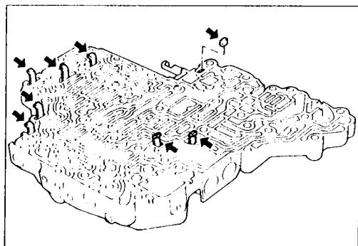
Check to see that retainer plates are properly positioned in lower body.
