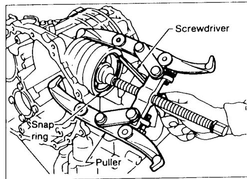
Remove band servo piston snap ring.
