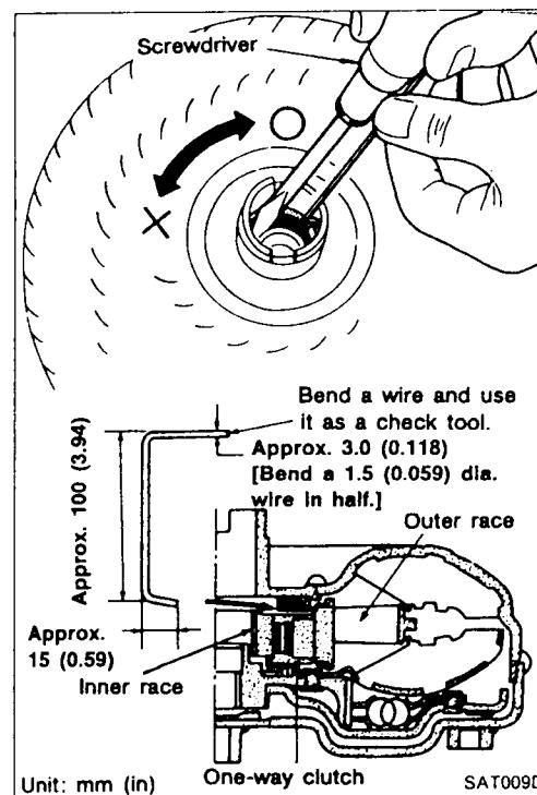
Check torque converter one-way clutch using check tool as shown at left.
