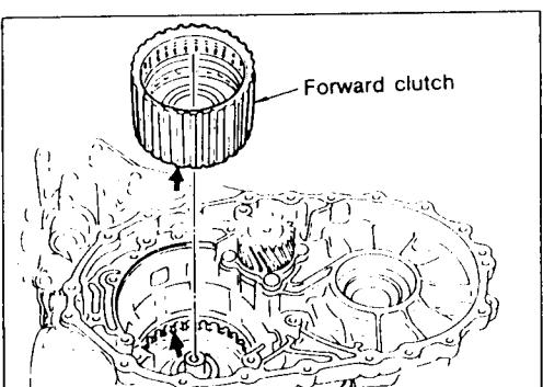
Remove forward clutch assembly from transmission case.
