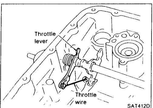
10. Install throttle wire to throttle lever.
