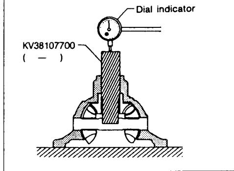
Measure clearance between side gear and
