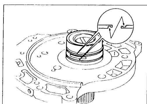
Install new seal rings carefully after packing ring groove with petroleum jelly and connect hooks.
