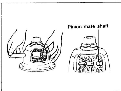
Install side gear and thrust washers in differential case.
