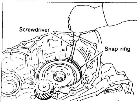
Remove snap ring using a screwdriver.
