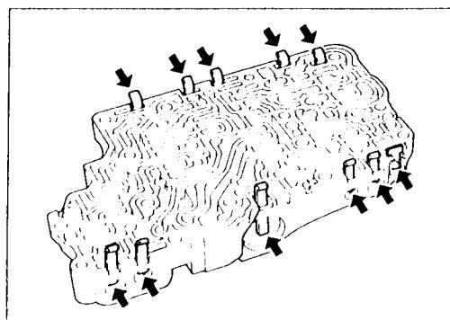
Remove valves at retainer plates.
