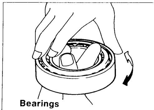
Make sure bearings roll freely and are free from noise, cracks, pitting or wear.
