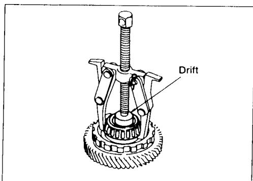
Remove idler gear bearing inner race.
