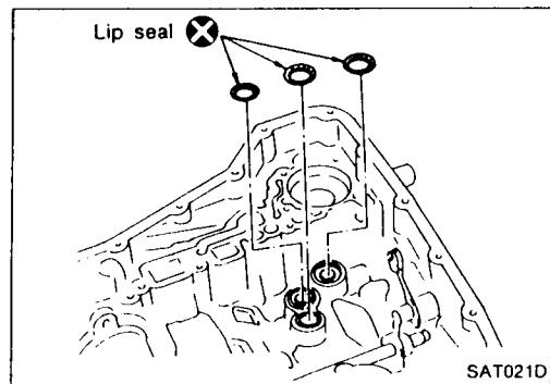
7. Install lip seals for band servo oil holes on transmission case.
