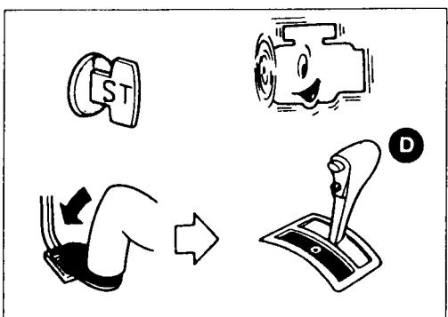
6. Accelerate to wide-open throttle gradually while applying foot brake.
