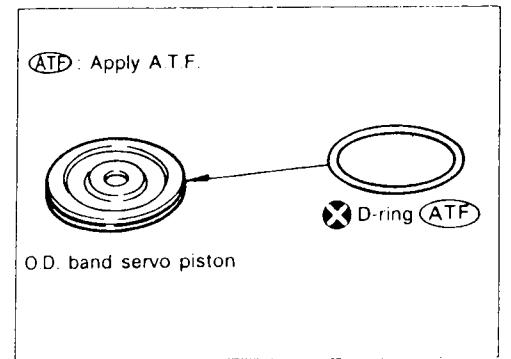
Install D-ring to O.D. band servo piston.
