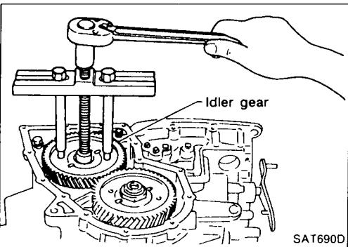
8. Remove idler gear to measure output shaft preload.
