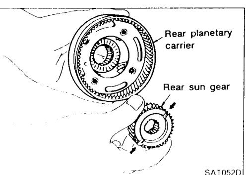
9. Install rear sun gear on rear planetary carrier.
