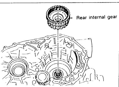
Remove rear internal gear from transmission case.
