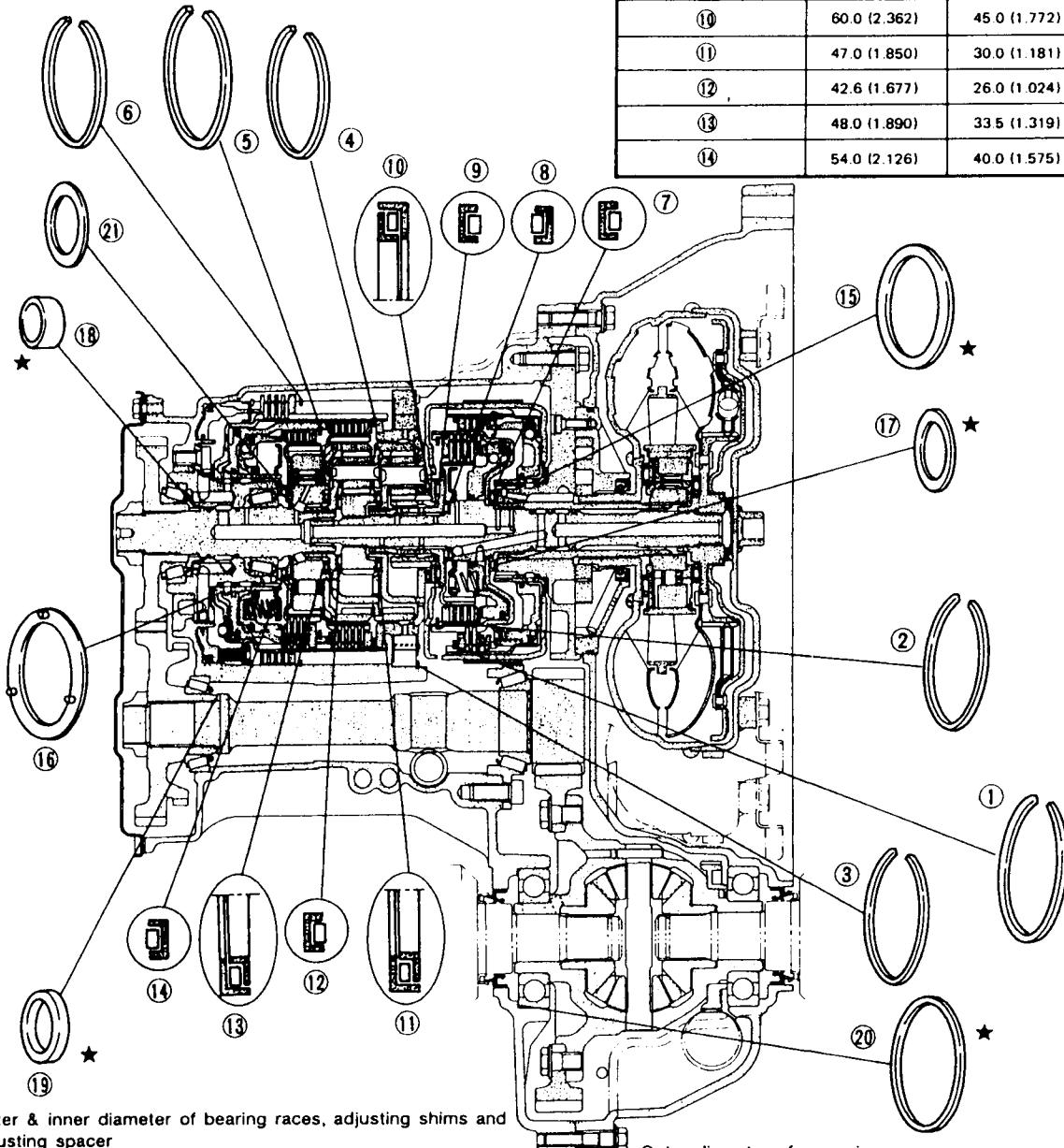
Outer & inner diameter of bearing races, adjusting shims and adjusting spacer
