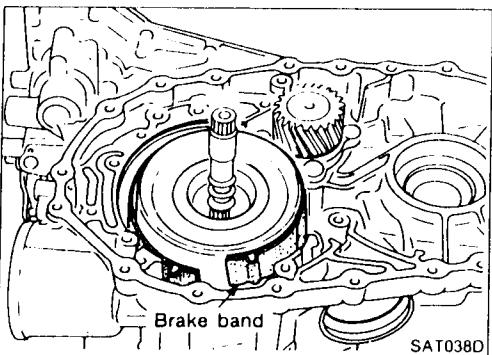
3. Install anchor end pin, washer and lock nut on transmission case.
