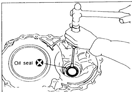
Remove oil seal from converter housing using a screw-driver.
