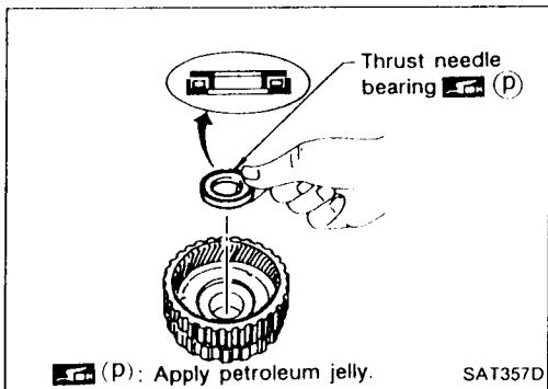
5. Install thrust needle bearing on rear internal gear.
