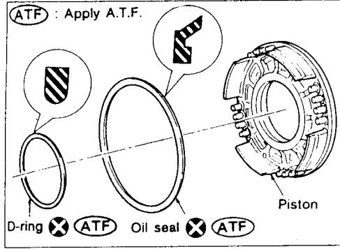
1. Install D-ring and oil seal on piston.
