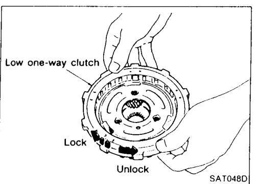
12. Install low one-way clutch to front planetary carrier by turning it in the direction of the arrow as shown.
