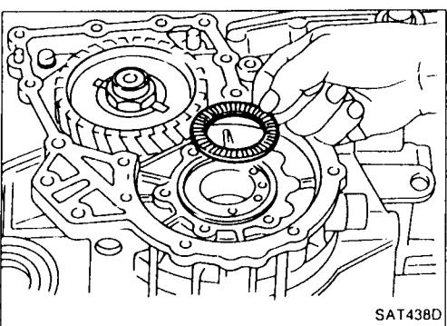
2. Install output shaft thrust needle bearing on bearing retainer.
