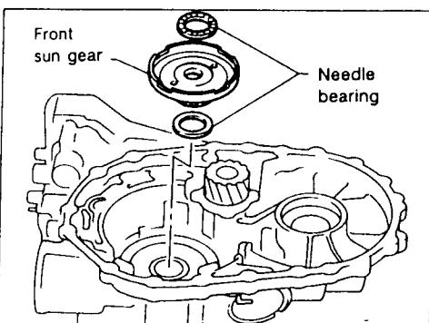
Remove front sun gear and needle bearings from transmission case.
