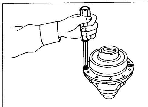
Install side gear (viscous coupling side) on differential case and then install viscous coupling.
