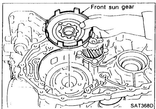
17. Install front sun gear on front planetary carrier.
