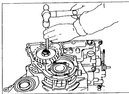
Unlock idler gear lock nut using a pin punch.
