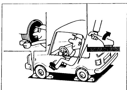
5. Start engine, apply foot brake, and place selector lever in "D" range.
