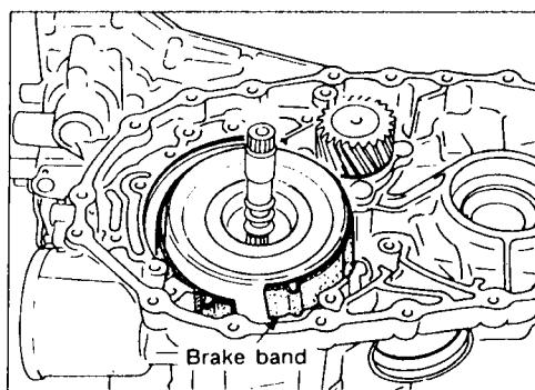
Remove brake band from transmission case.
