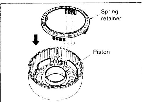
Install return springs and spring retainer on piston.
