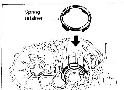
**Install return springs and spring retainer on piston.**
