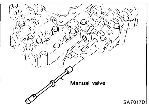
11. Install control valve assembly.
