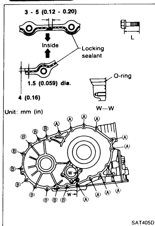
4. Install O-ring on differential oil port of transmission case.
