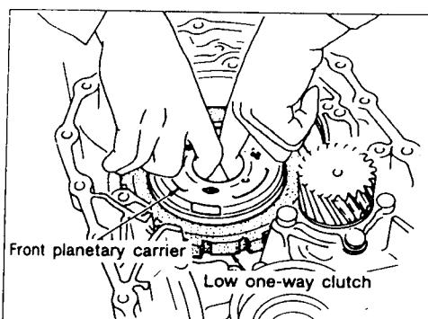
Remove front planetary carrier with low one-way clutch.
