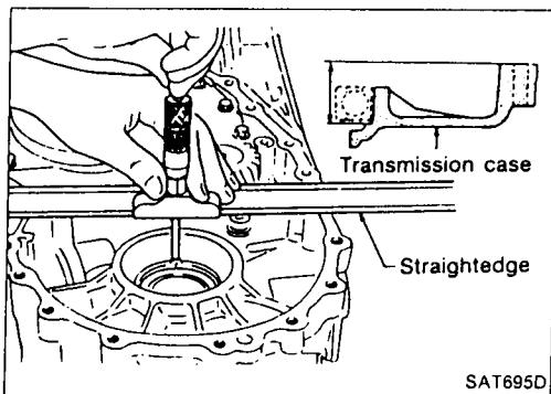
1. Measure dimension "T" between side bearing fitting surface of transmission case and converter housing fitting surface of transmission case.
