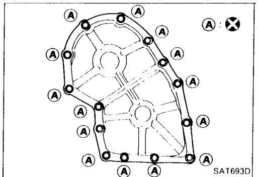
12. Install new gasket and side cover on transmission case.
