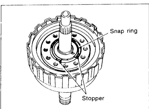
**Do not align snap ring gap with spring retainer stopper.**
