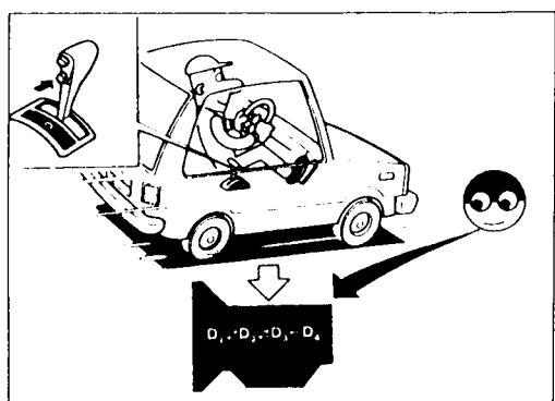
4. Check to determine if shifting to overdrive gear cannot be made while O.D. control switch is "OFF".
