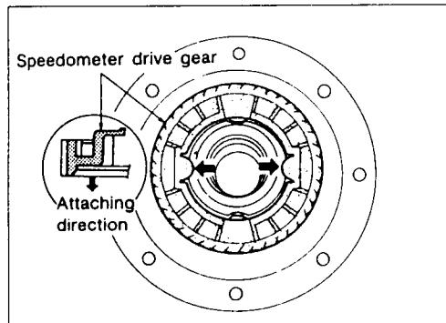
Align the projection of speedometer drive gear with the groove of differential case.
