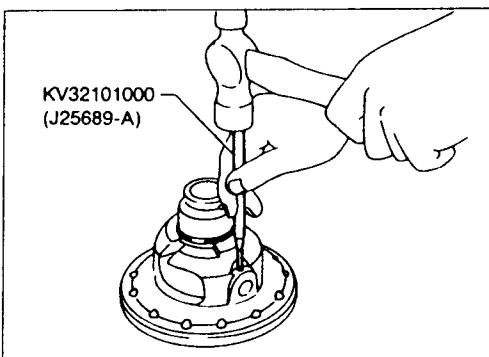
Install retaining pin.
