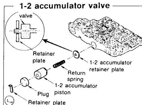
Install 1-2 accumulator valve and then align 1-2 accumulator retainer plate with 1-2 accumulator valve from opposite side of control valve body.
