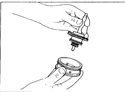
Install band servo piston assembly to servo piston retainer by pushing it inward.
