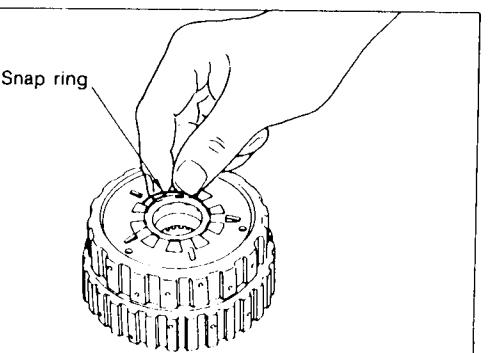
Install snap ring to groove of rear internal gear.
