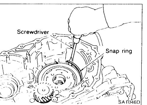
15. Install snap ring with screwdriver.
