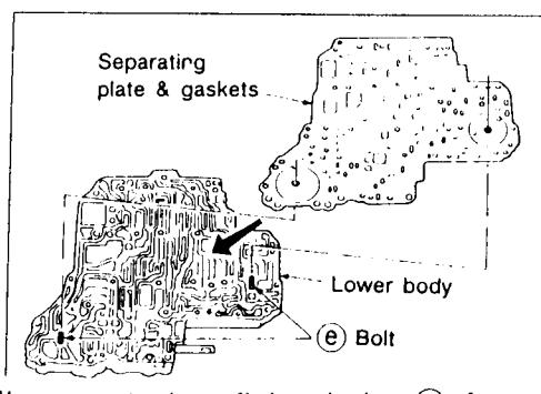
Install support plate fixing bolts ② from bottom of lower body and install separating gaskets and separating plate as a set on lower body using bolts ③ as guides.
