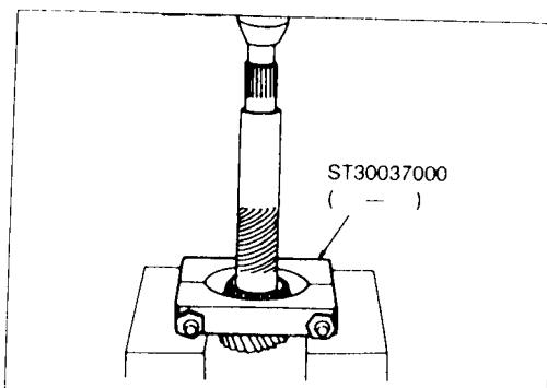
Press out reduction gear inner race from reduction gear.
