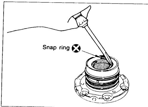
Install snap ring to bearing retainer.
