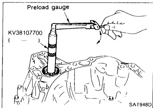
14. Insert Tool into differential case and measure turning torque of final drive assembly.
