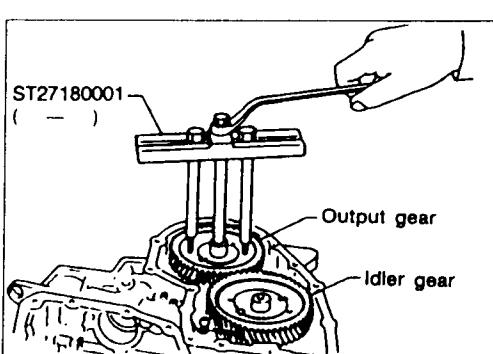
Remove idler gear and output gear using a puller.
