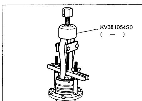
3 Remove output shaft bearing outer race from bearing retainer.
