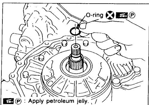
Remove oil pump according to the following procedures. Remove O-ring from input shaft.
