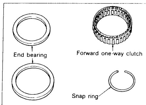
Check snap ring and end bearings for deformation damage.
