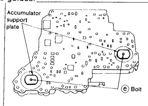
Temporarily install support plates on lower body.
