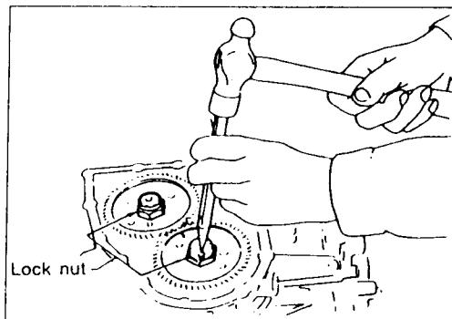
Unlock both idler gear and output gear lock nuts using a pin punch.
