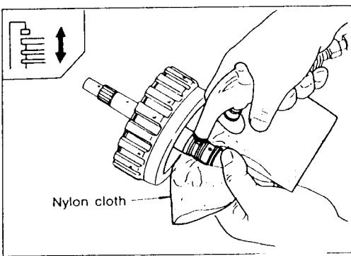
Check operation of high clutch.
