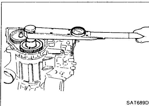
7. Tighten output gear lock nut to specified torque.
