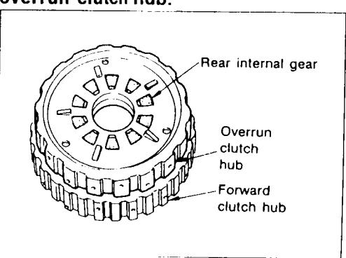
Install overrun clutch hub on rear internal gear.
