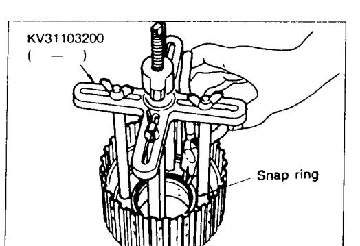
Install overrun clutch piston assembly on forward clutch piston while turning it slowly.
