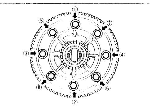
Install final gear and tighten fixing bolts in numerical order.
