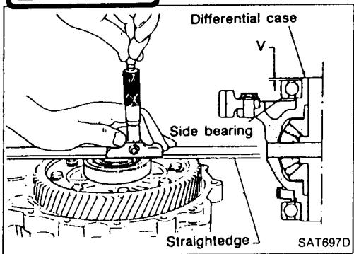
5. Measure dimension "V" between end of differential case and adjusting shim mating surface of differential side bearing.
