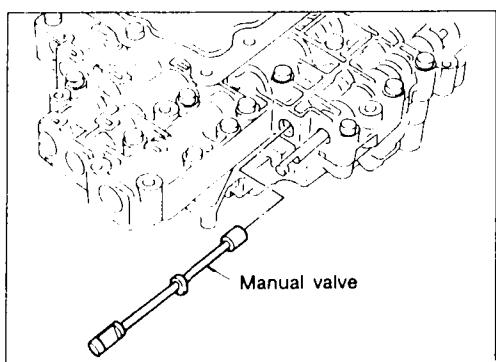
10 Remove manual valve from control valve assembly as a precaution.
