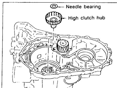
Remove high clutch hub and needle bearing from transmission case.
