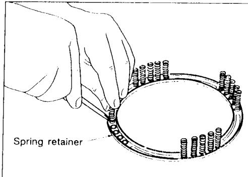
**Do not remove return springs from spring retainer.**
