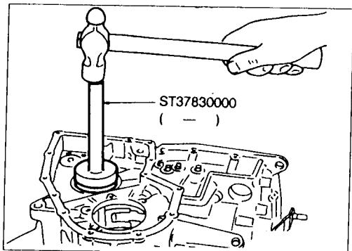
Install idler gear bearing outer race on transmission case.
