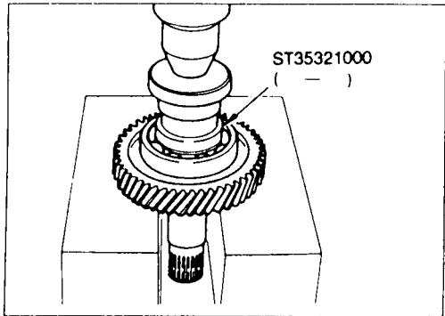
Press output shaft bearing on output shaft.
