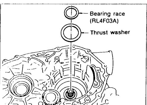
Remove thrust washer and bearing race from transmission case. (only RL4F03A)
