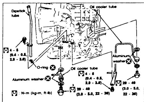
Remove oil charging pipe and oil cooler tube.
