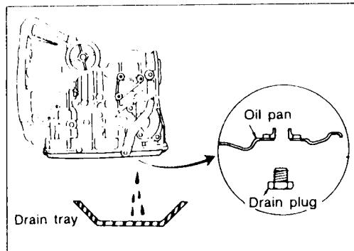
Drain A.T.F. through drain plug.
