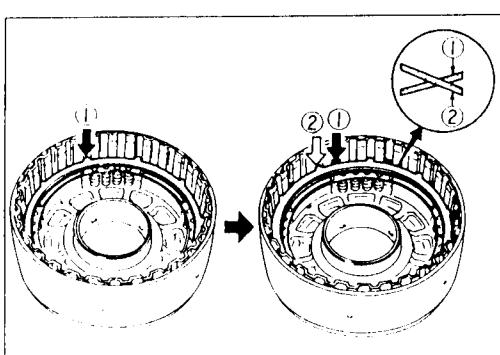
Do not align the projections of any two dish plates.
