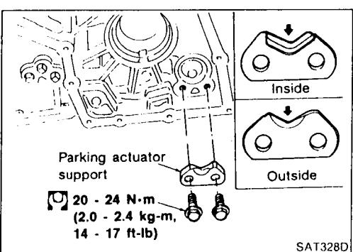
2. Install parking actuator support to transmission case.
