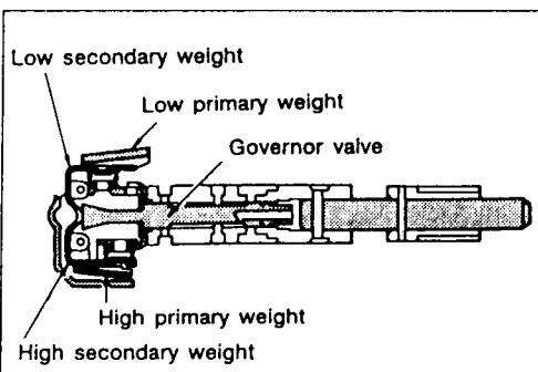
With low primary weight closed, place top of governor valve assembly down to make sure governor valve proper lowers under its own weight.
