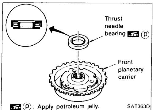
11. Install thrust needle bearing on front planetary carrier.
