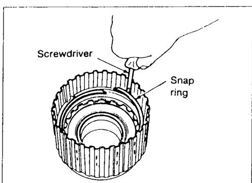
Install snap ring for overrun clutch.
