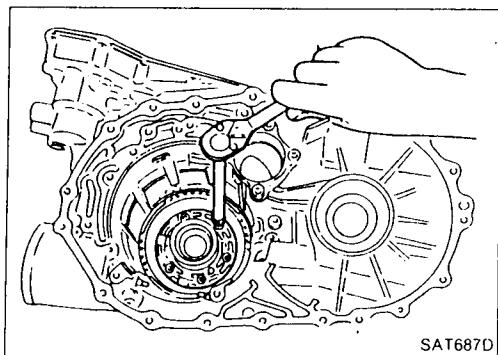
2. Install bearing retainer on transmission case.
