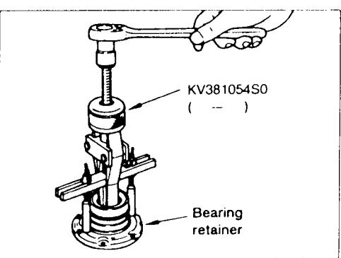
Remove needle bearing from bearing retainer.
