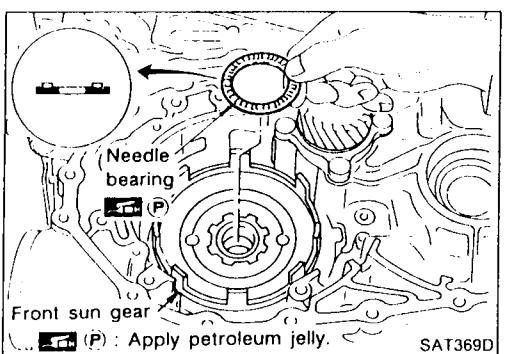
18. Install needle bearing on front sun gear.
