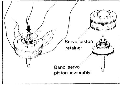
Remove band servo piston assembly from servo piston retainer by pushing it forward.
