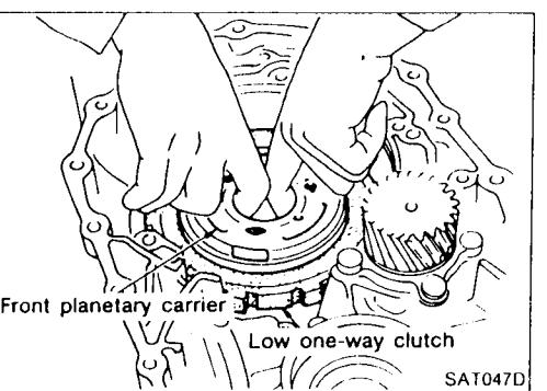
14. Install front planetary carrier assembly on transmission case.
