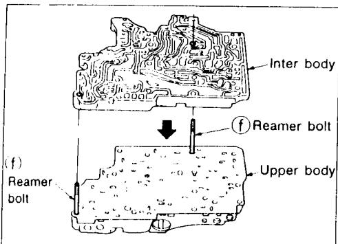
Install inter body on upper body using reamer bolts ① as guides.
