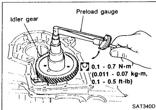
7. Measure turning torque of reduction gear.
