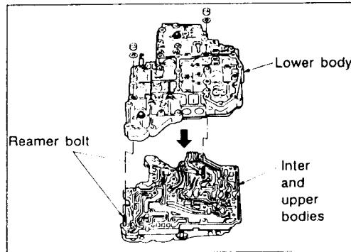
Install lower body on inter body using reamer bolts ① as guides and tighten reamer bolts ① slightly.
