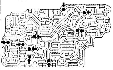
Check to see that steel balls are properly positioned in upper body and then remove them from upper body.
