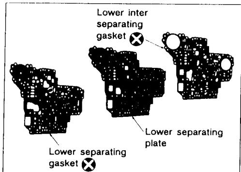
Install lower separating gasket, inter separating gasket and lower separating plate in order shown.
