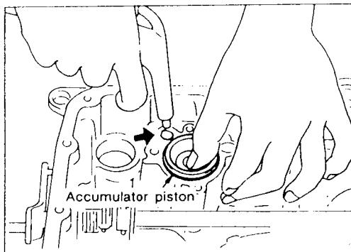
13 Remove N-D accumulator piston and return spring with compressed air.
