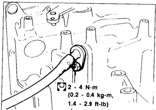
18 Remove throttle wire mounting bolt.
