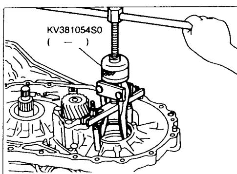
23 Remove differential side bearing outer race from transmission case (RL4F03V).
