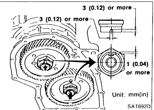
10. Install idler gear and tighten lock nut to specified torque.
