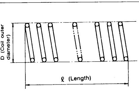
**Oil cooler relief valve spring.**
