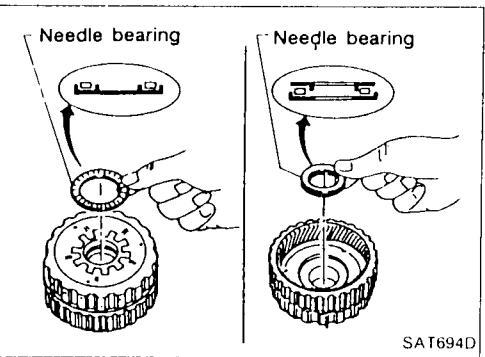
5. Install needle bearings on rear internal gear.
