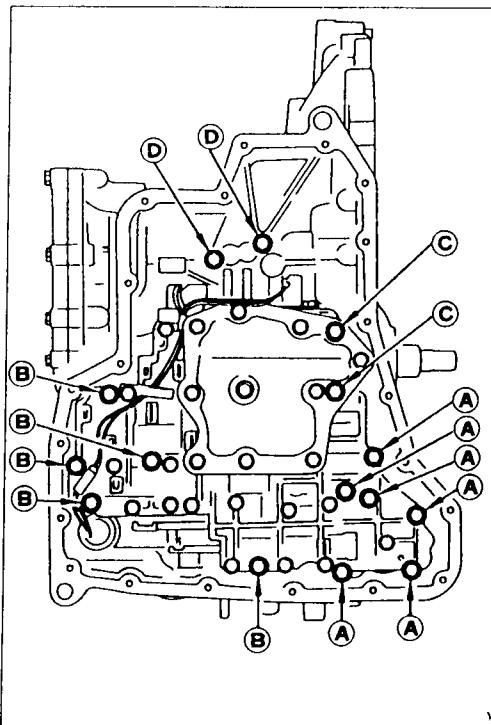
Remove control valve assembly according to the following procedures.
