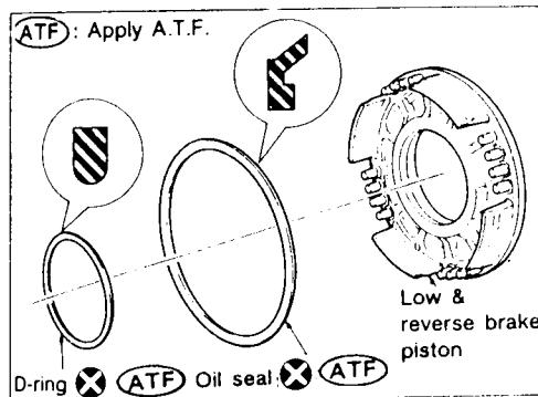
Install D-ring and oil seal on piston.
