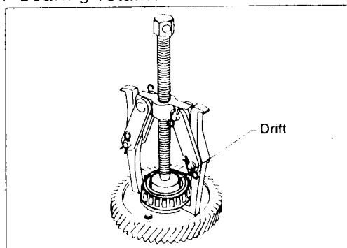
4 Remove output gear bearing inner race.
