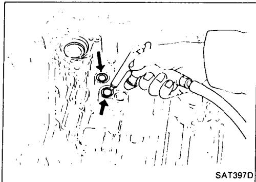
11. Apply compressed air to oil holes of transmission case and check operation of brake band.
