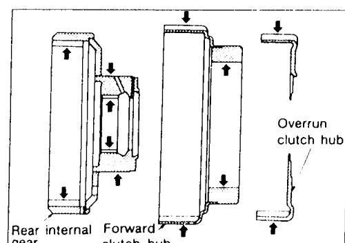
Check rubbing surface for wear or damage.
