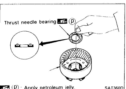
8. Install needle bearing on rear planetary carrier.
