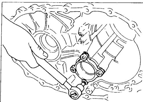
Remove reduction gear bearing outer race from transmission case.
