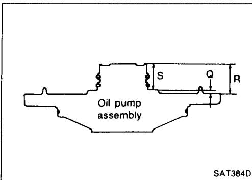
2. Measure dimensions "R" and "S" and then calculate dimension "Q".
