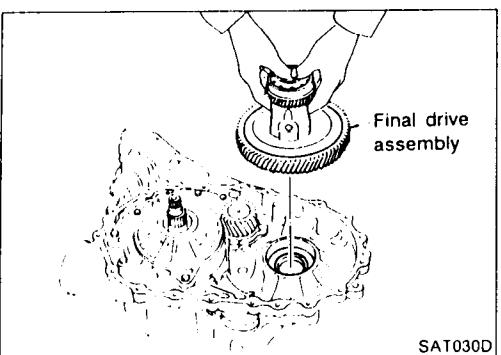
2. Install final drive assembly on transmission case.
