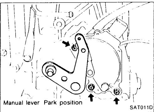
14. Install inhibitor switch.
