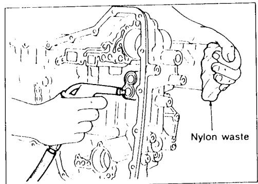
Apply compressed air to oil hole in transmission case to remove O.D. servo piston retainer and band servo piston assembly.
