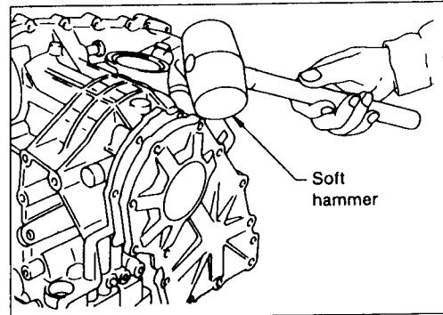
Remove side cover by lightly tapping it with a soft hammer.
