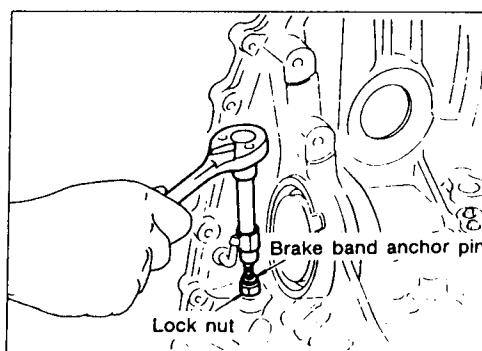
Remove brake band according to the following procedures.
