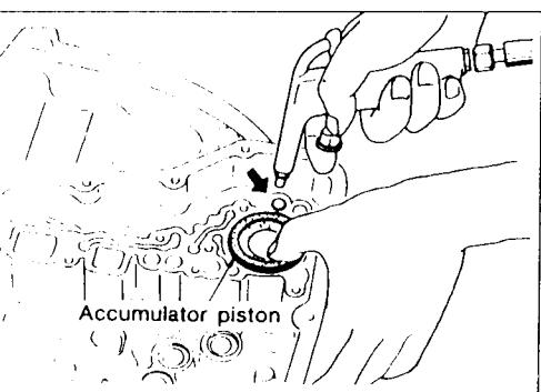
12 Remove 3-R accumulator piston with compressed air.
