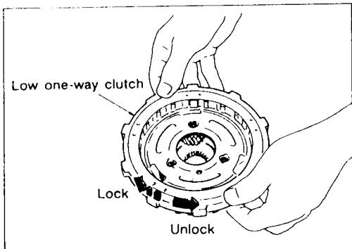
Check that low one-way clutch rotates in the direction of the arrow and locks in the opposite direction.
