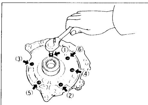
Loosen bolts in numerical order and remove oil pump cover.
