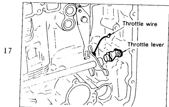
17 Remove throttle wire from throttle lever.
