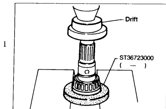
1 Press out output shaft bearing inner race.
