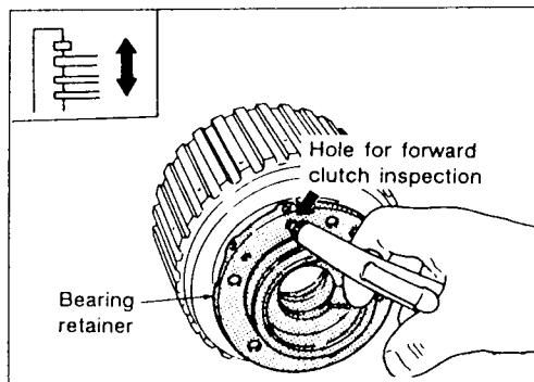
Check operation of forward clutch.
