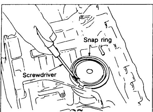
Remove snap ring using a screwdriver.
