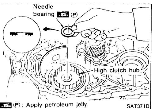
20. Install needle bearing on high clutch hub.
