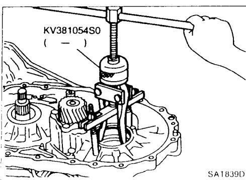
9. Remove converter housing from transmission case.
