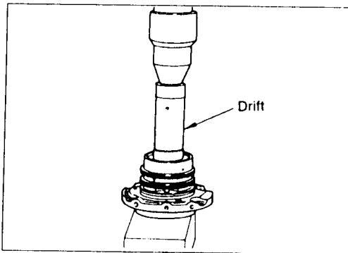
Press needle bearing on bearing retainer.
