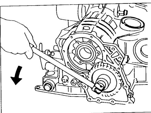
Remove idler gear lock nut.
