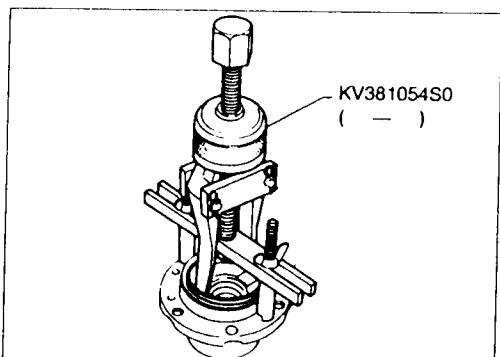
Remove output gear bearing outer race from bearing.
