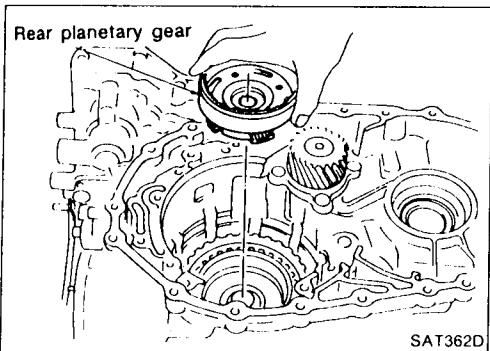
10. Install rear planetary carrier on transmission case.
