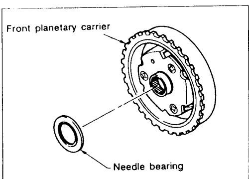
Remove needle bearing from front planetary carrier.
