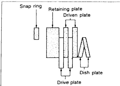
Install drive plates, driven plates, retaining plate and dish plates.
