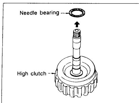
Remove needle bearing from high clutch drum.
