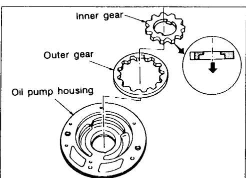
Remove inner and outer gear from oil pump housing.
