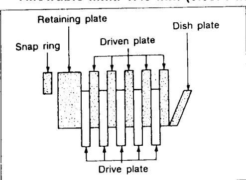
Install drive plates, driven plates, retaining plate and dish plate for forward clutch.
