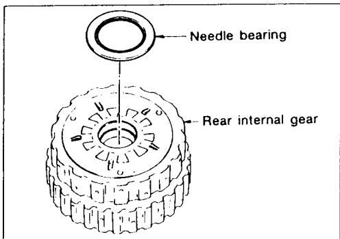
Remove needle bearing from rear internal gear.
