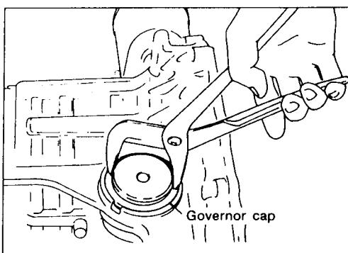
Remove governor cap using water pump pliers.
