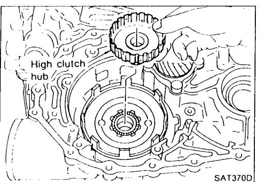
19. Install high clutch hub on front sun gear.
