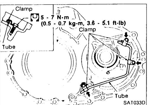
3. Install oil tube on converter housing.
