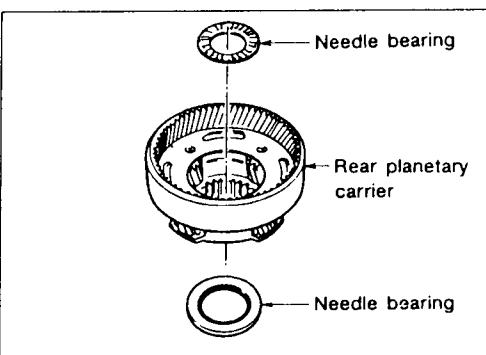
Remove needle bearings from rear planetary carrier assembly.
