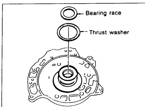
Remove thrust washer and bearing race from oil pump assembly.
