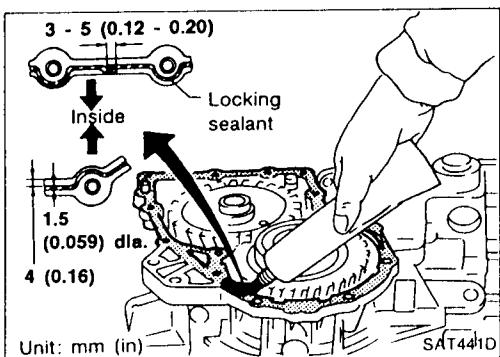
8. Apply locking sealant to transmission case as shown in illustration.
