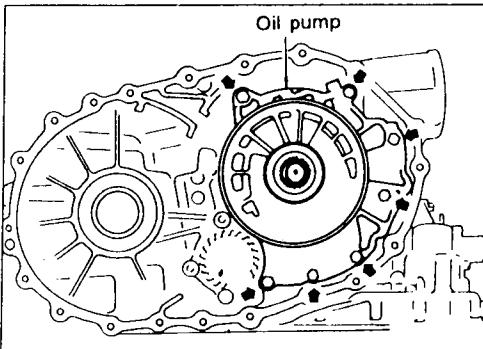
Remove oil pump assembly from transmission case.
