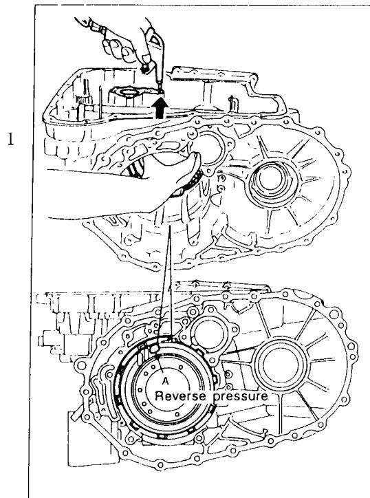
Apply compressed air to oil hole of transmission case while holding piston.
