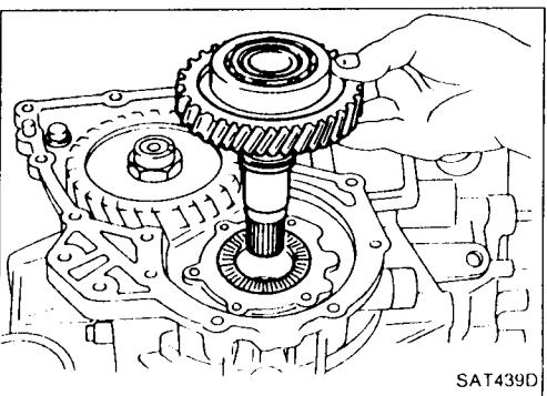
3. Install output shaft on transmission case.
