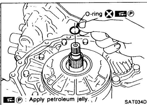
9. Install O-ring to input shaft.
