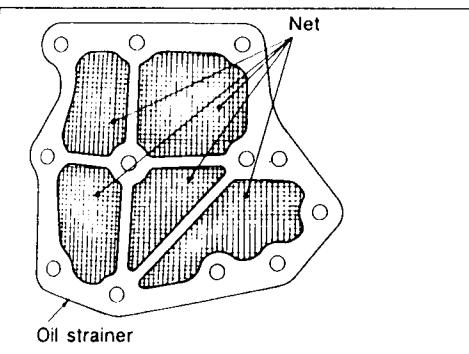
Check wire netting of oil strainer for damage.
