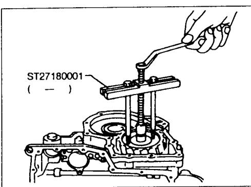
Remove idler gear with puller.
