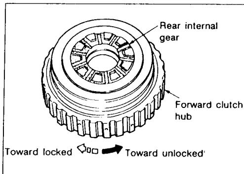
Install forward clutch hub on rear internal gear.
