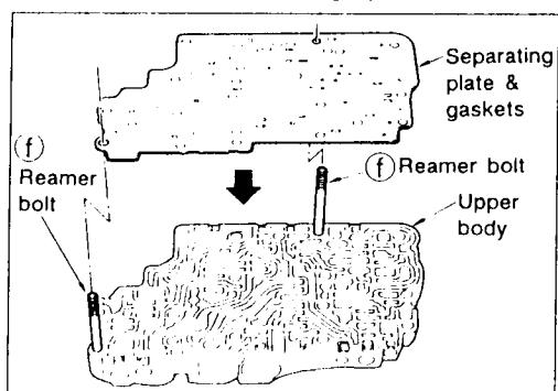
Install reamer bolts ① from bottom of upper body and install separating gaskets and separating plate as a set on upper body using reamer bolts as guides.
