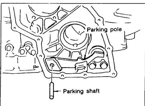
Draw out parking shaft and remove parking pole from transmission case.
