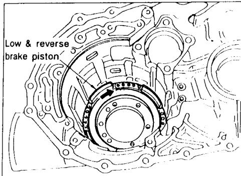
**Install piston assembly on transmission case while turning it slowly.**
