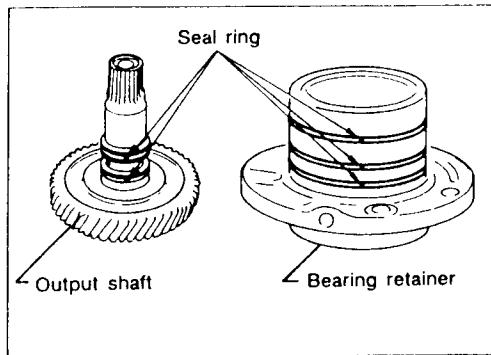
Install new seal rings to output shaft and bearing retainer carefully
