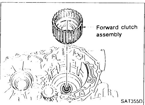
3. Install forward clutch assembly.
