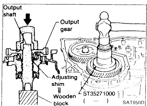
3. Place output shaft on bearing retainer.
