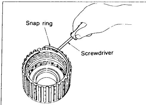
Install snap ring for forward clutch.
