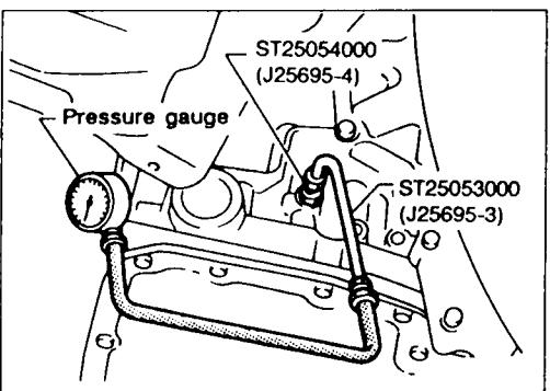
3. Install pressure gauge to line pressure port.
