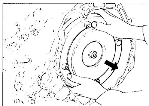
Remove torque converter.
