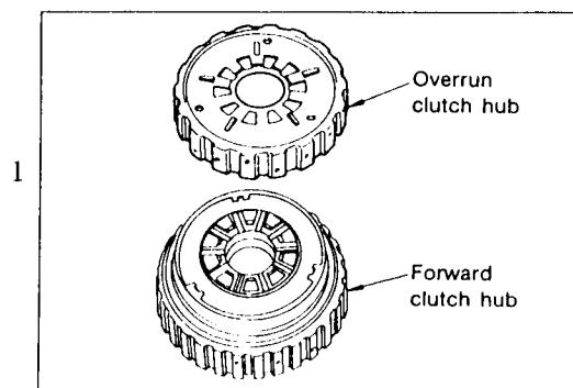
Remove overrun clutch hub from forward clutch hub.
