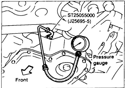
3. Install pressure gauge to governor pressure port.
