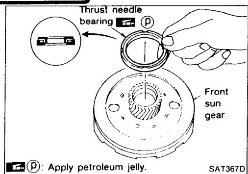
16. Install needle bearing on front sun gear.
