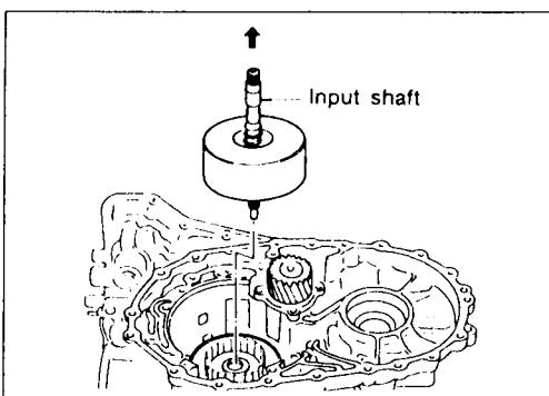
Remove input shaft assembly (high clutch) with reverse clutch.
