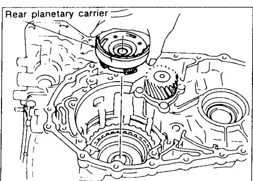
Remove rear planetary carrier assembly from transmission case.
