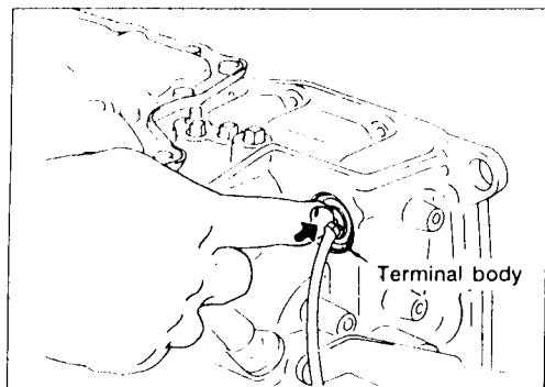
9 Push terminal body into transmission case and draw out solenoid harness.
