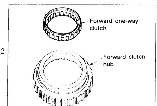
Remove one-way clutch from forward clutch hub.
