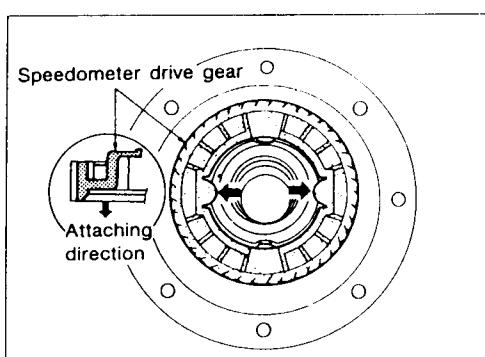
Install retaining pin.
