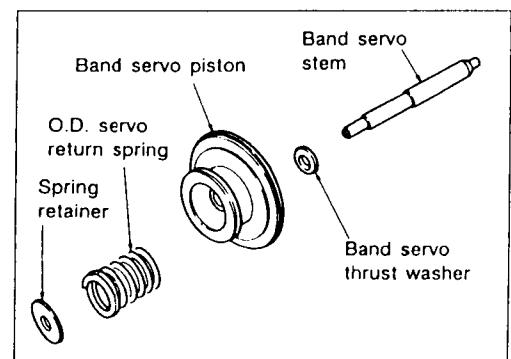
Install band servo piston stem, band servo thrust washer, O.D. servo return spring and spring retainer to band servo piston.
