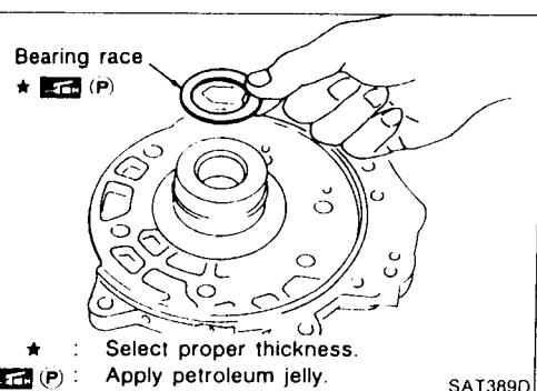
5. Place bearing race selected in total end play adjustment step on oil pump cover.
