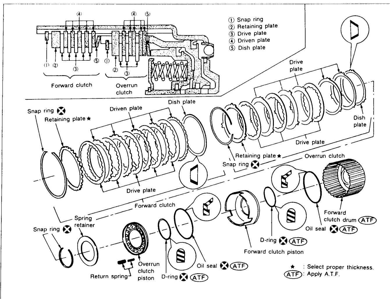
**Forward clutch and overrun clutch return springs**
